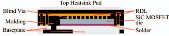
Fig. 1. The cross-section of SiC MOSFET FOPLP.
