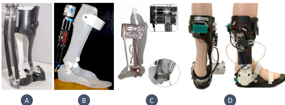
Figure 8: (A) Active AFO with two pneumatic artificial muscles, (B) Active AFO with series elastic actuator, (C) Insertion Point Eccentricity Controlled (IPEC) AFO, (D) Design of a compact high-torque actuation system for portable powered ankle-foot orthosis.
