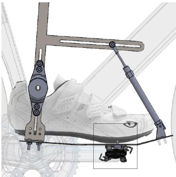
Figure 77: shows the envisioned set-up for a functional prototype; a regular cycling shoe used which is bolted onto the baseplate, subsequently the baseplate is sandwiched between the cycling shoe and an SPD mounting bracket which can be (dis)mounted onto the Shimano SPD pedal.
