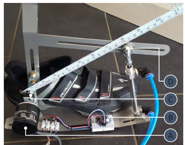
Figure 98: Allocation of (A) rotary encoder, (B) gyro sensor, (C) joint axis, and (D) cylinder piston anchor point.
