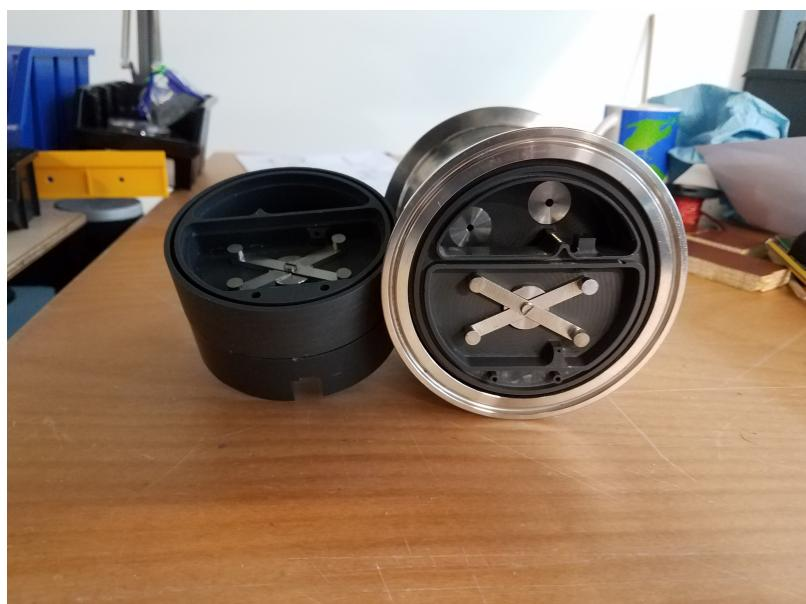
Figure G.6. Frontal view of both sides of electrolysis cell.
