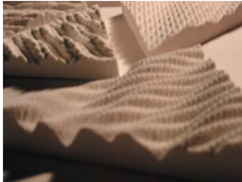
Figure 5. Computer generated concrete free-form object.
