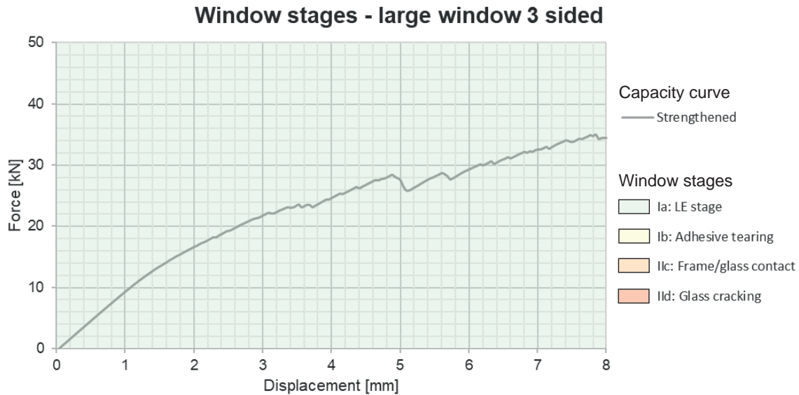
Figure 13.20: Projection of the window substages on the capacity curve of the strengthened URM wall with a large window 3 sided.
