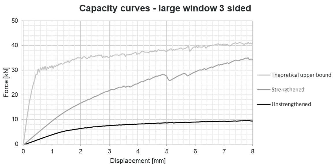
Figure 13.19: Capacity curves of seismic strengthening predictions for the URM wall with a large window 3 sided.
