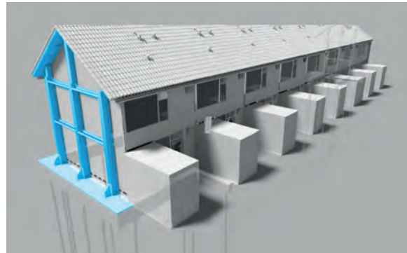
Figure 5.2: Strengthening of terraced houses in longitudinal direction with a steel frame inside the cavity [9] or a steel supporting structure at the end wall. [10]
