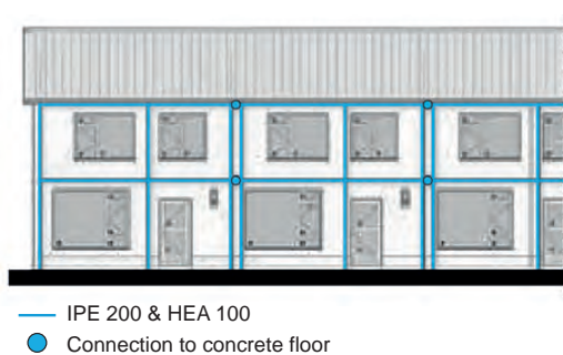
Figure 1.4: Strengthening of terraced houses in longitudinal direction with a steel frame inside the cavity [9] or a steel supporting structure at the end wall. [10]
