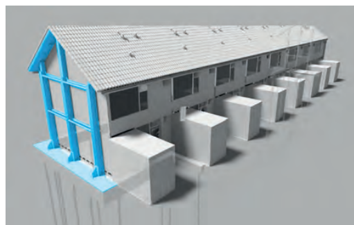
Figure 1.4: Strengthening of terraced houses in longitudinal direction with a steel frame inside the cavity [9] or a steel supporting structure at the end wall. [10]
