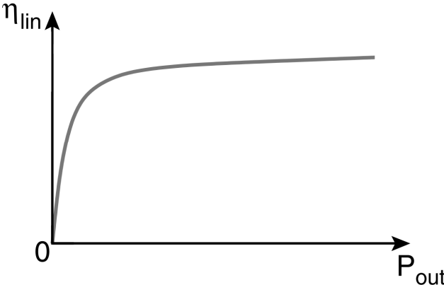
Figure 15 Typical efficiency curve of a DC/DC converter [29]
