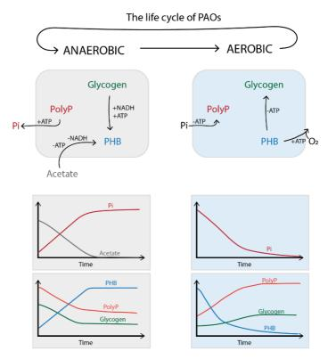
**Figure 4**. A typical cycle of PAOs in EBPR systems. In this schematic, the dynamic changes of extracellular and intracellular components that a typical PAO cell experiences during an EBPR cycle are represented.
