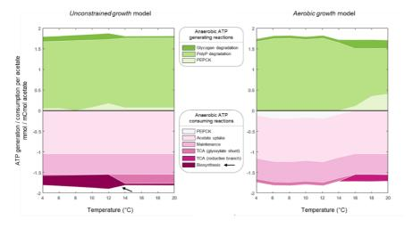
**Figure 4**. Balance and reactions involved in the ATP generation (green) and consumption (magenta) during the anaerobic phase of the PAOs simulations at different temperatures of the unconstrained growth (left panel) model and the aerobic growth(right panel) model. Black arrow indicates the use of ATP for biosynthetic reactions showcasing the main difference in the structure between both
