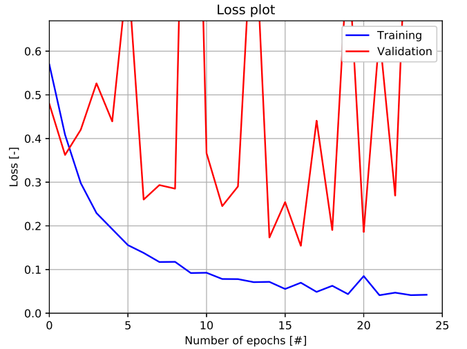
Fig. 17: Loss plot R_o = 0.7 for different random data split.
