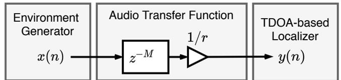
Fig. 2: The main components of an audio-based localization simulator using TDOA. Input audio signal  $x(n)$  is delayed by  $z^{-M}$  representing  $M$  samples, attenuation is represented by  $1/r$  ( $r$  being distance) and the result is a time-discrete signal  $y(n)$ .
