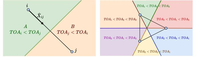
(a) Perpendicular bisector cutting the plane of possible beacon locations in half based on TOA. (b) Sections created by the CTP algorithm when three microphones are uniformly distributed around a circle.
