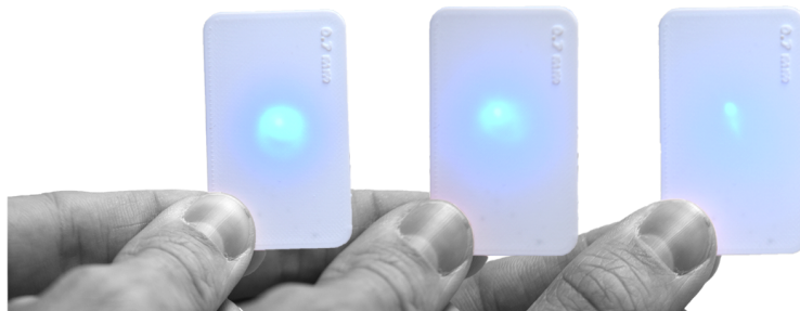
Figure 2: 0.7 mm PLA with different distances to the led (left to right: 10mm, 20mm, 30mm)
