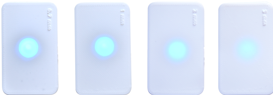
Figure 5: LED through different PLA thicknesses (left to right: 0.7mm, 1mm, 2mm, 3mm)
