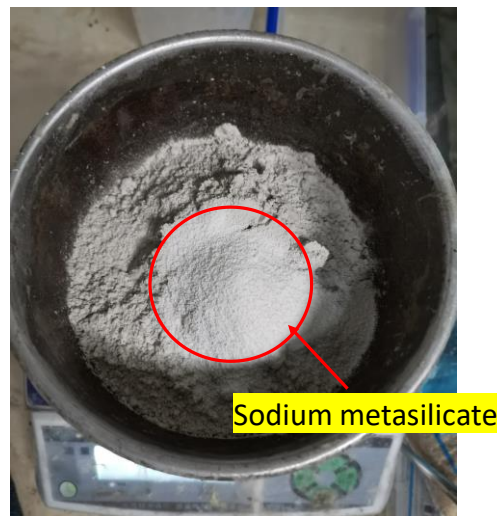
Fig. 2. Direct addition of sodium metasilicate particles into the dry mixture (GBFS + sand) prior to the addition of distilled water into the system.
