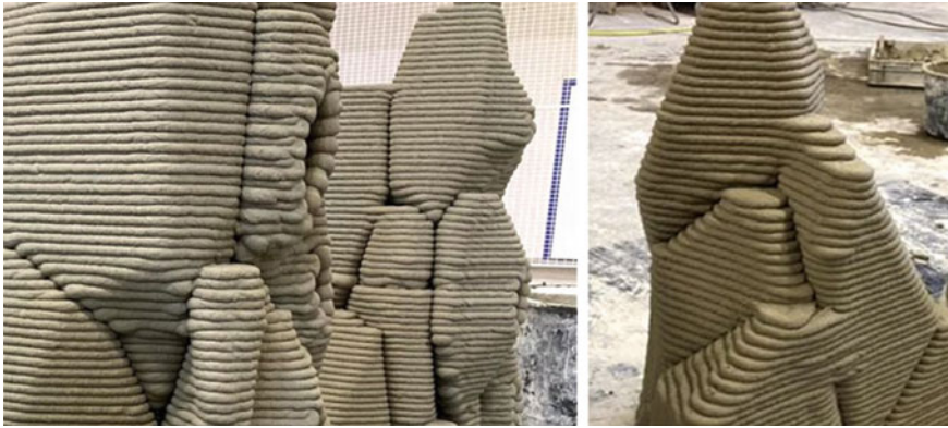
Fig. 3.6 Stackable 3D printed components
