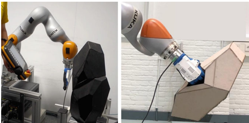
Fig. 3.3 Rhizome 1.0 component mockups and HRI-supported assembly test
