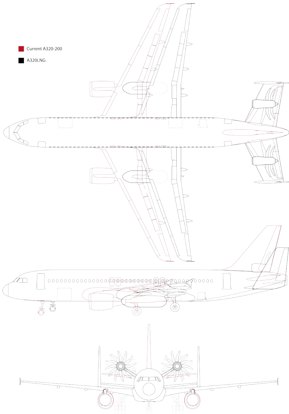
Figure 22-5: 3 views of the changes in configuration between the A320 and the A320-LNG
