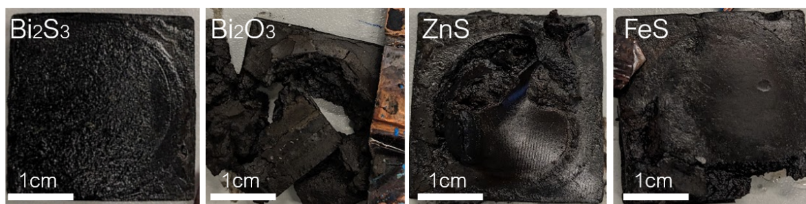
Figure 5.32: Overview of left A) bismuth sulfide B) bismuth oxide C) zinc sulfide and D) iron sulfide after durability test in the half cell.
