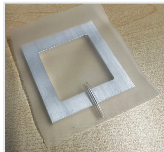
Figure 5.14: PU tube placed on top of PU ply
