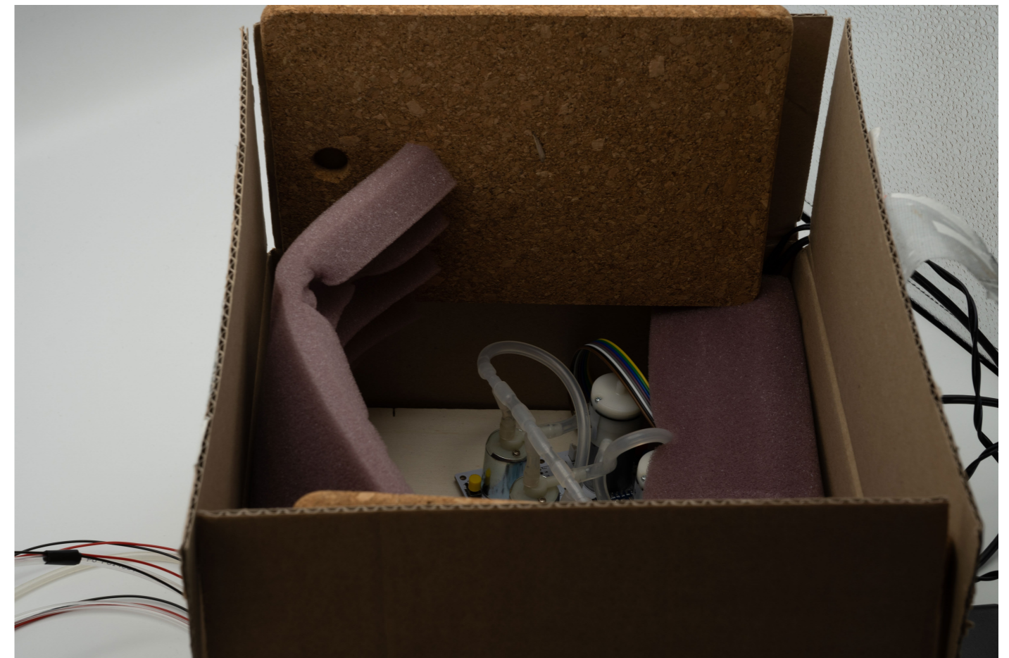
Figure 5.36: Soundproofing box for the pumps and valves 67
