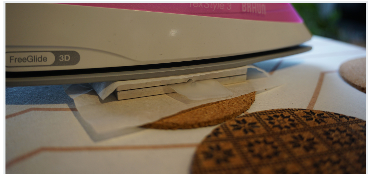
Figure 5.13: Heating aluminum mold to create an airtight seal around the nozzle
