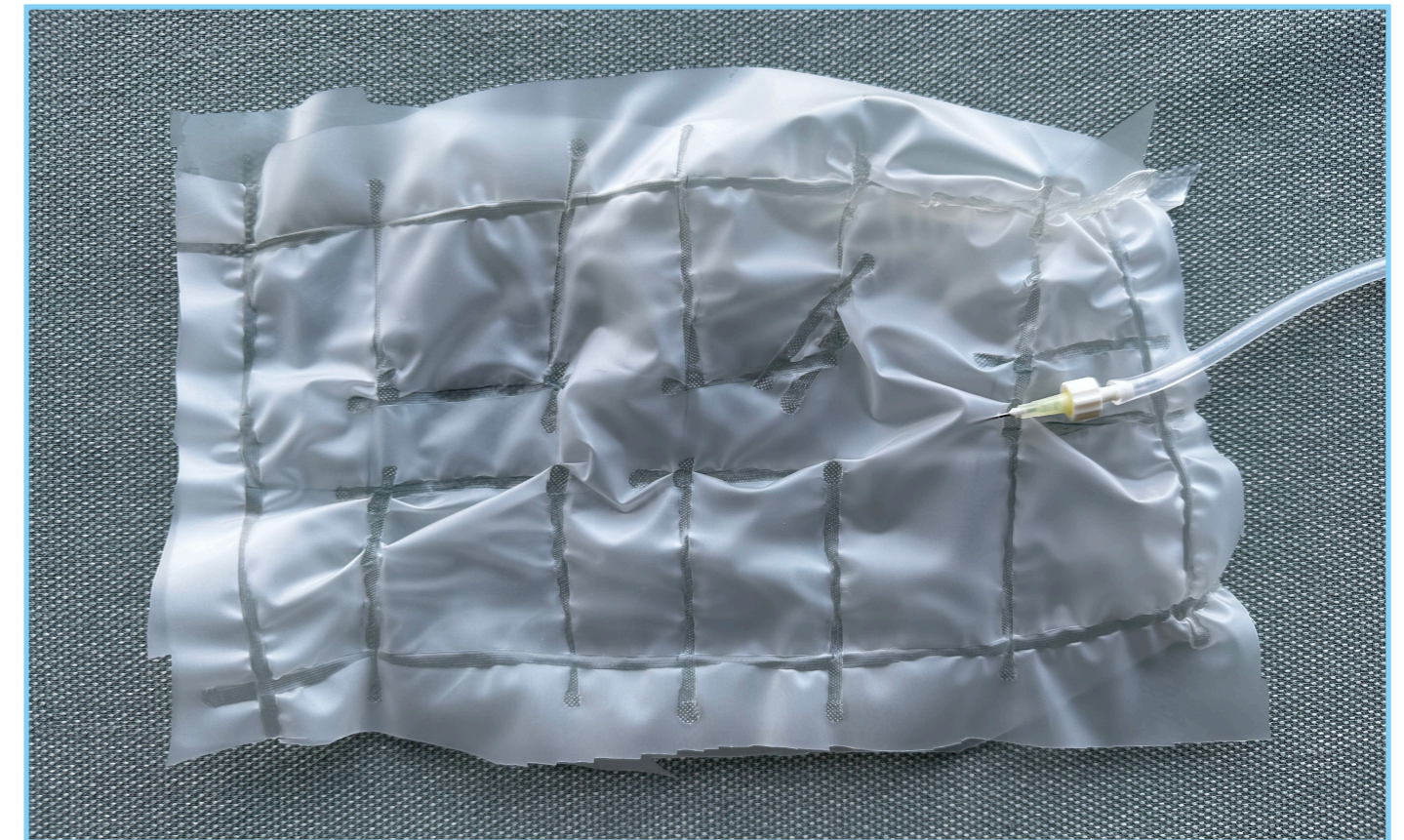
Figure 5.17: Failed prototype trying to embed a 'stroke' actuation within the airbag design
