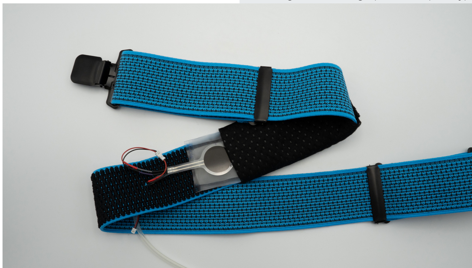
Figure 2.2: Overview of textile-integrated actuator and sensor
