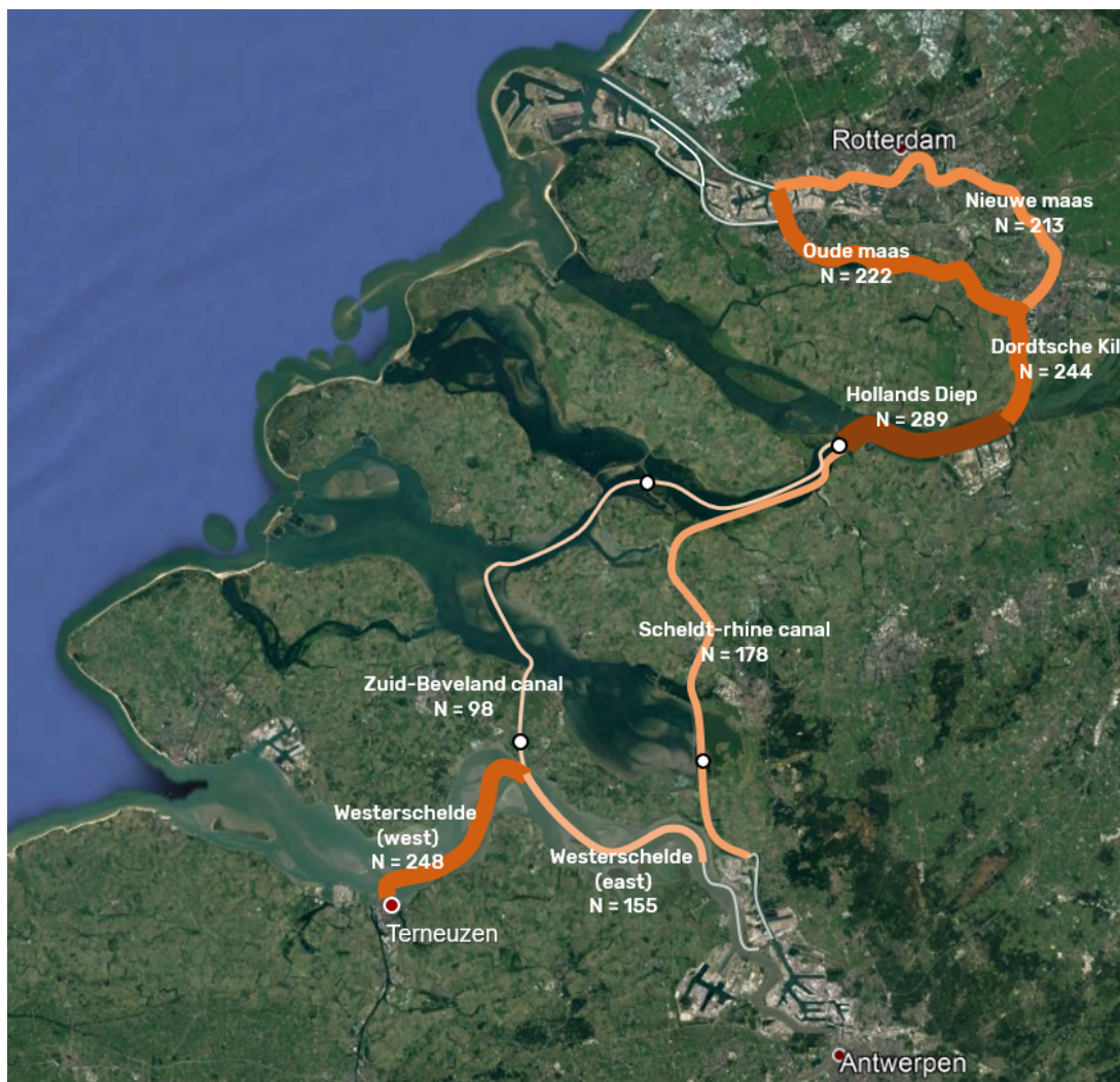
Figure 5.14: Traffic intensity on the Rotterdam-Antwerp corridor, based on an AIS dataset of one day (2 September 2019)
