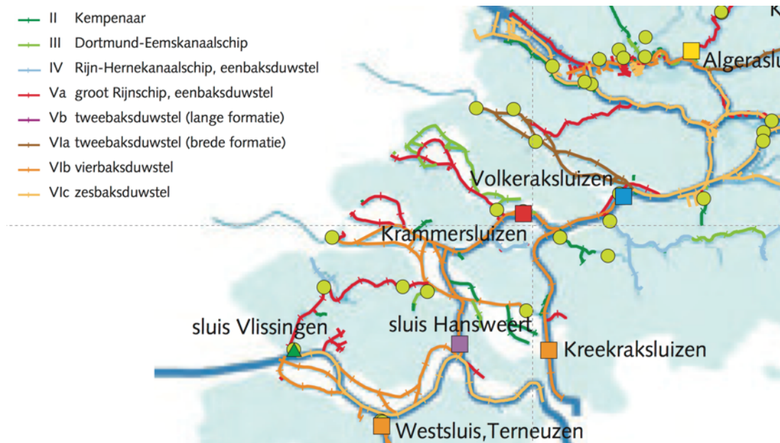
Figure 5.6: Specified CEMT class of each waterway section on the Rotterdam-Antwerp corridor (Rijkswaterstaat, 2009)
