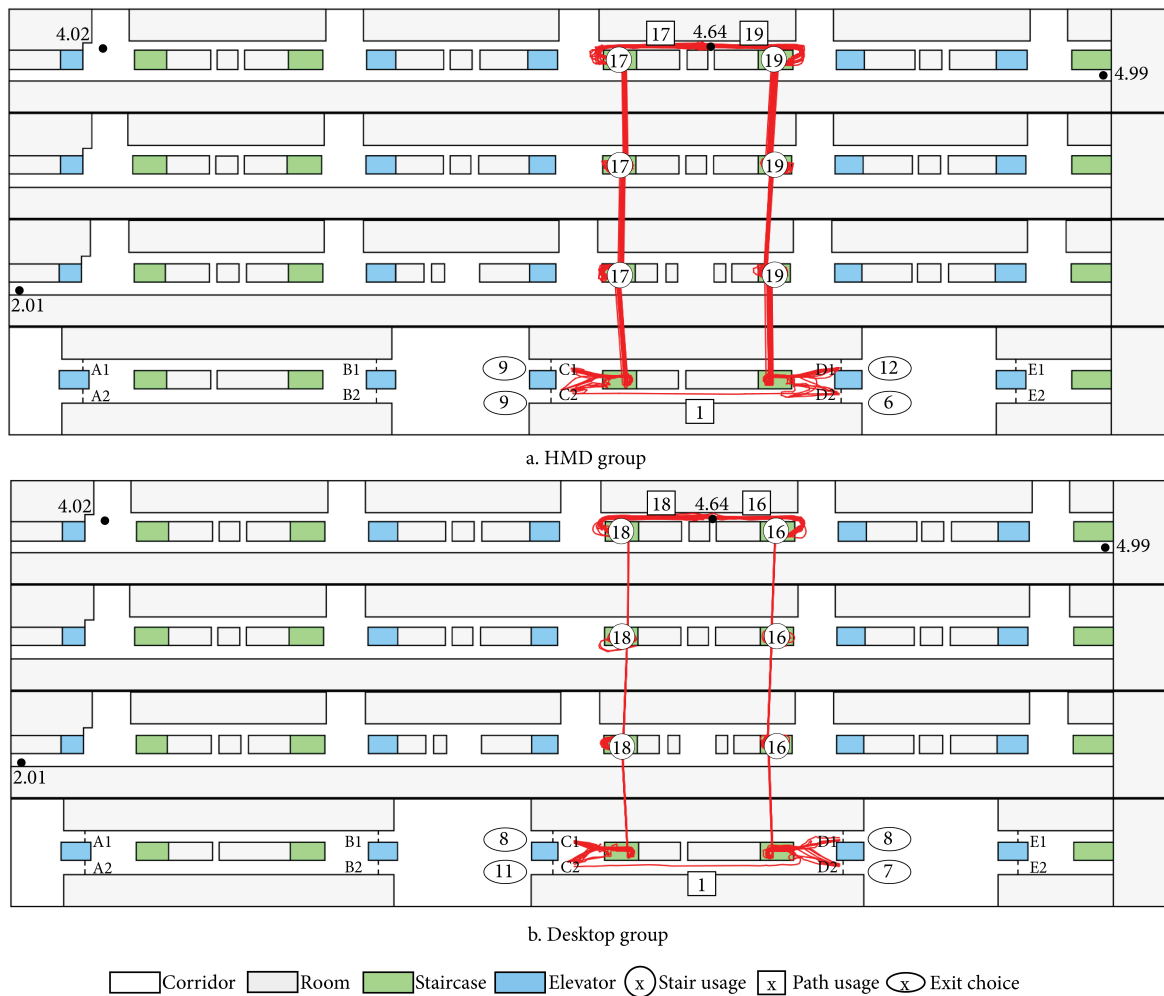
Figure 5. 11: Visualisation of the participants’ movement trajectories and the frequency of staircase, path, decision point and evacuation exit usage during task 4.
