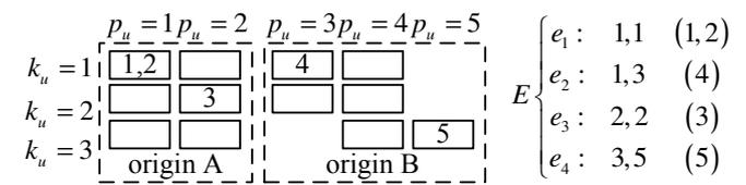
Fig. 2. Example of a created evacuation scheme. Groups 1,2 and 3 belonging to origin A and groups 4 and 5 belonging to origin B are assigned to elements (combinations of departure times 1, 2 and 3 and routes 1, 2, 3, 4 and 5). Evacuation scheme  $E$  contains four instructions (i.e.  $e_1$  containing  $k_e = 1$  and  $p_e = 1$  where groups 1 and 2 are assigned to).
