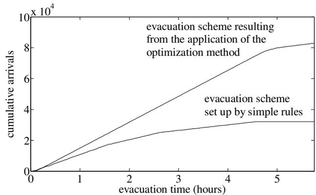
Fig. 6. Arrival pattern of the evacuation by applying the approximation of the optimal evacuation scheme and the evacuation scheme set up by simple rules.
