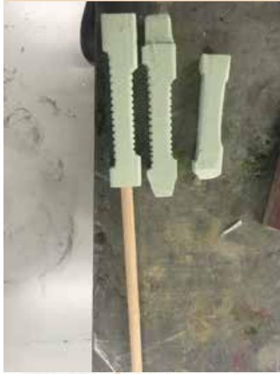
5. The cane parts are milled out of beechwood. Three parts are milled to allow for two bands.
