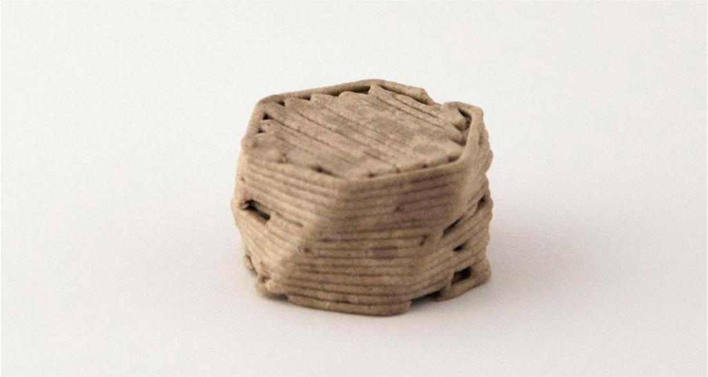
Figure 5.4. Result of material extrusion with recycled material.
