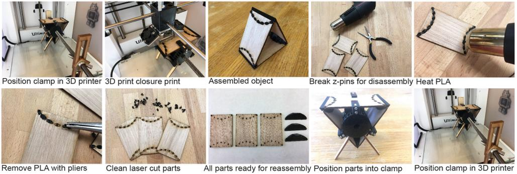
Figure 4.7. Assembly, disassembly and reassembly of the prism
