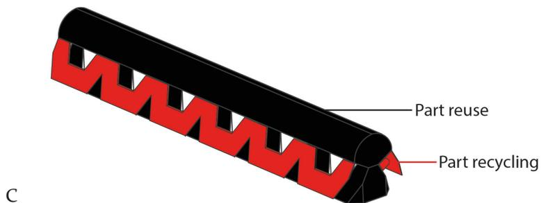
Figure 7.2. A: procedure to create reversible joint. B: parts are fixed in a clamp for assembly by 3D printing. C: Part of joint suitable for reuse (black) and recycling (red).
