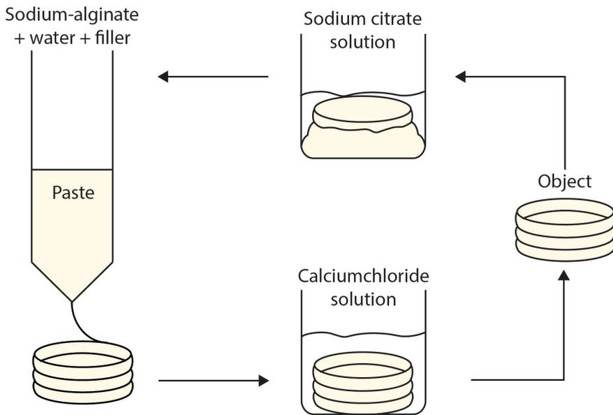
Figure 6.3. (Re)printability process based on ion cross-linking
