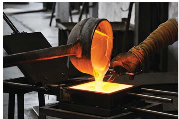
Figure 4.9 The process of casting glass. Source: (F Oikonomopoulou, Veer, Nijse, & Baardolf, 2014)
