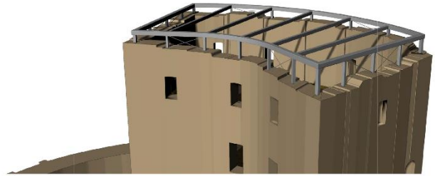
Step 1: Steel contour frame
