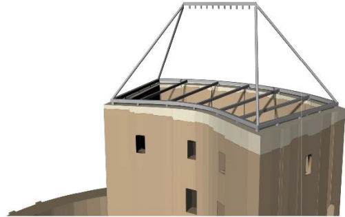
Step 3: Steel side and top profiles
