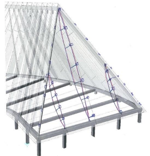
Figure 6.18 3D impression of the side trusses. Source: own ill.
