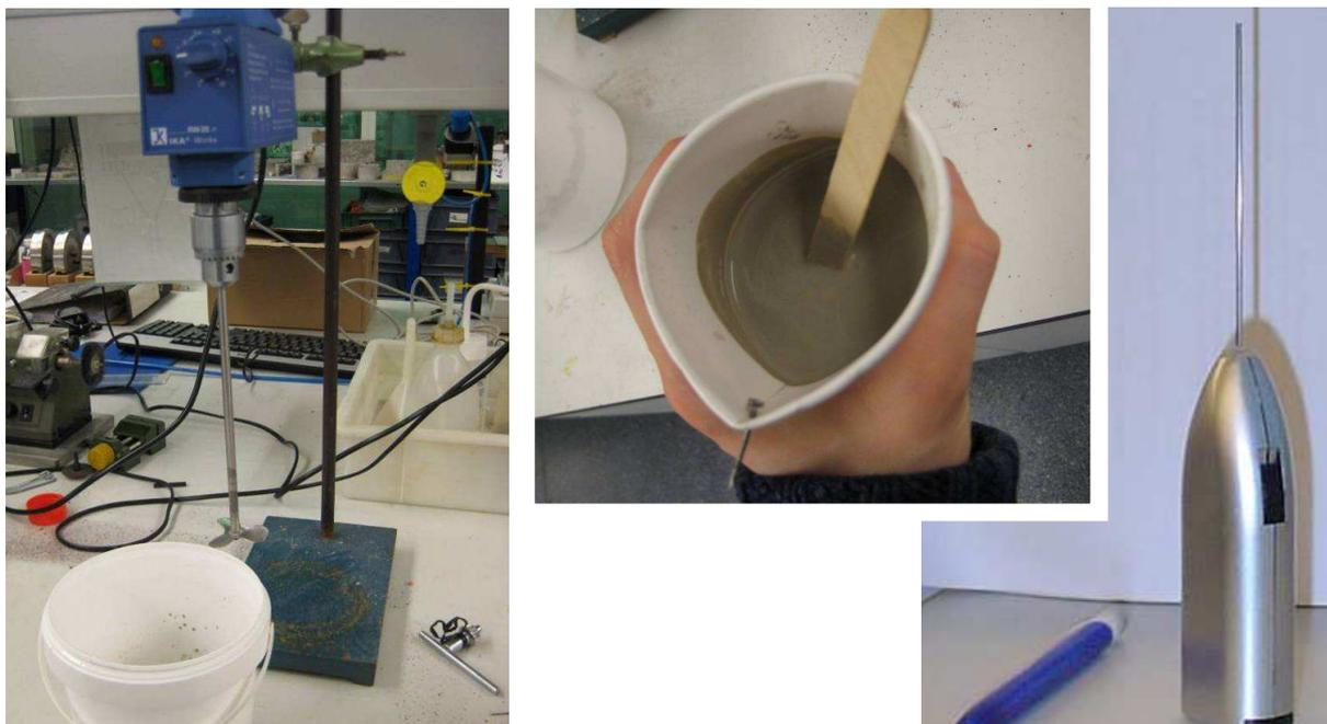
Figure 21 Paste production: Mixing device (l), cup for pouring (m), vibrating device (r)
