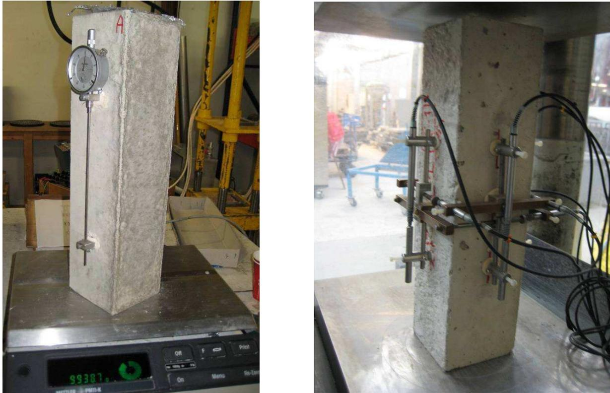
**Figure 22** Test for shrinkage with “clocks” (l) and modulus of elasticity (r)
