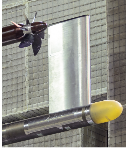
Figure 3. Pylon model installed upstream of the APIAN propeller model.
