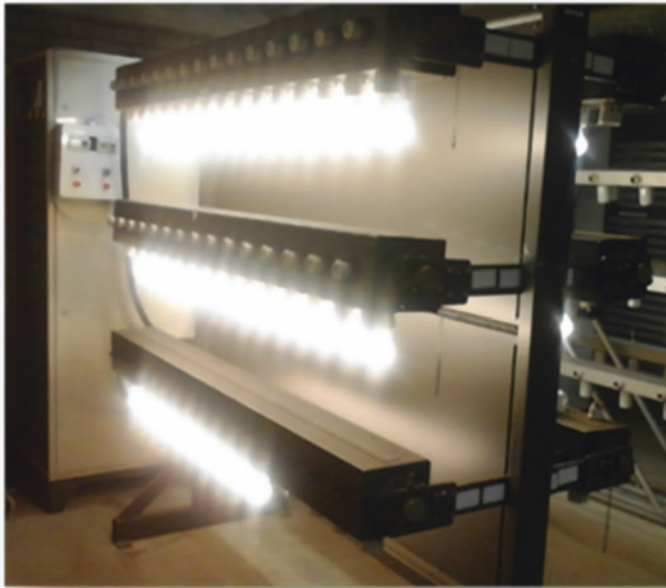
Fig. 7.12 Lifetime tests with glass LED bulbs put into traditional burning racks
