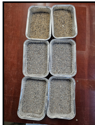
d) Materials after the oven drying The 2 in the top are sand, the 2 in the Middle are Milled fRCA, and the 2 in the bottom are fRCA
