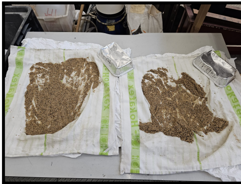
b) Materials left to dry till SSD condition The 2 in the left are sand, the 2 in the Middle are Milled fRCA, and the 2 in the right are fRCA
