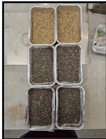
c) Materials before the oven drying The 2 in the top are sand, the 2 in the Middle are Milled fRCA, and the 2 in the bottom are fRCA
