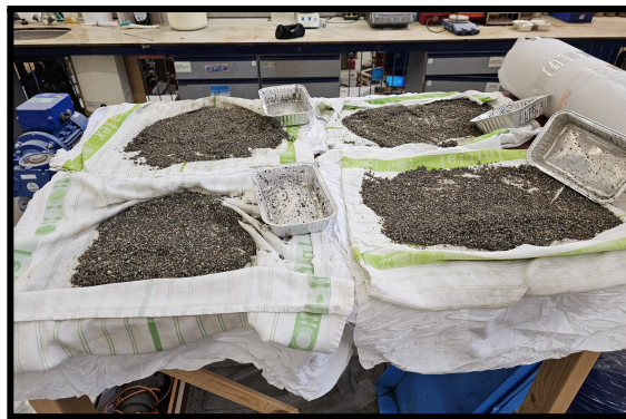
b) Materials left to dry till SSD condition The 2 in the left are sand, the 2 in the Middle are Milled fRCA, and the 2 in the right are fRCA
