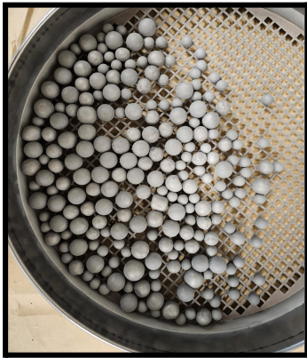
Figure 4.2: Steel balls used for milling
