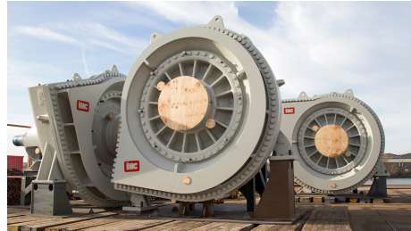
Figure 1.2: Dredge pump typical dimensions are 3 [m] and a power of 5 [MW].
