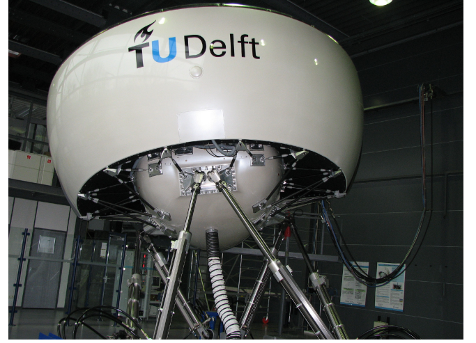
Fig. 6. SIMONA Research Simulator (SRS) using a Stewart platform as moving base simulator. [22]
