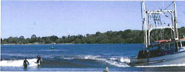
Figure 3. River testing such as that shown in this figure has proven that even the smallest of pressure source generated waves can be consistently surfed. (Reproduced with permission of Liquid Time Pty Ltd).
