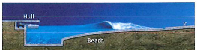
Figure 1. Concept design for the efficient method of generating continuously surfable breaking waves using moving pressure sources. (Reproduced with permission of Liquid Time Pty).
