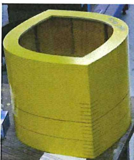
Figure 10. Model 2 parabolic pressure source of 700mm length, 600mm beam, 500mm height.
