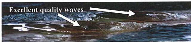
Figure 12. Examples of excellent waves generated in the circular scale model by model 10 with d^* = 0.2 in h_0 = 250\text{mm} at Fr_{h0} = 0.975 .
