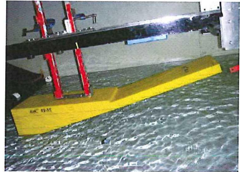
Figure 11. The first wavedozer shape Model 3 tested. The direction of travel was from left to right.
