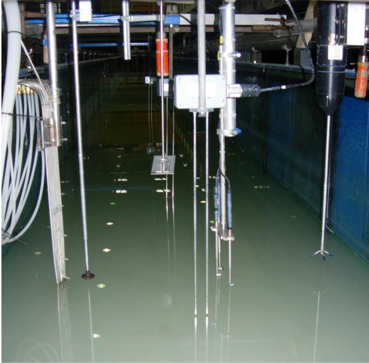
Figure 2.8 From left to right: TSS, EMS, reference rod, WHM, ASTM, ADV
