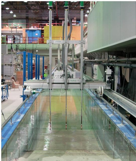
Figure 2.6 Bed profiler with three probes
