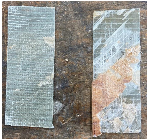
Fig. 4.6: Difference in delamination between inside (left, cohesive failure) and outside laminate (right, mixed failure).
