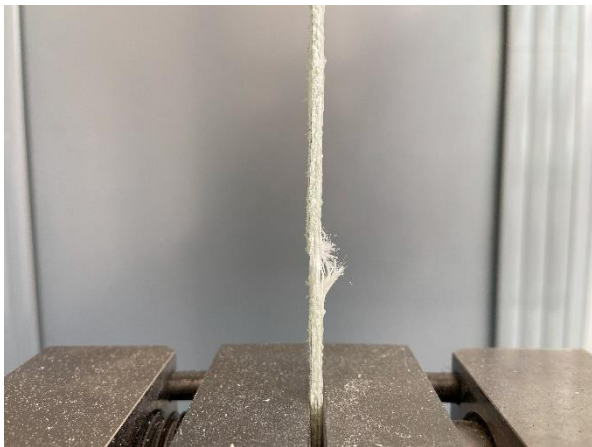
Fig 5.7: A torn GRP specimen
