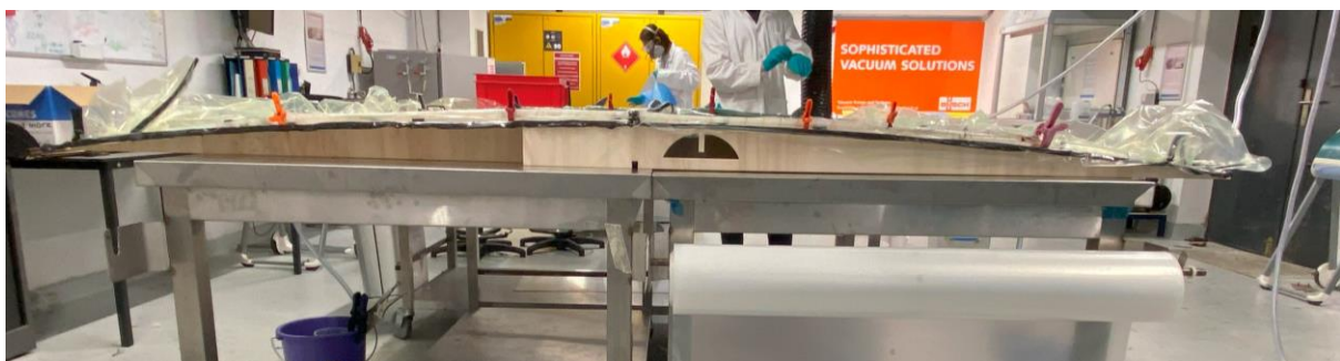
Fig. 8.3: Bulkhead supporting the shape of the mould.
