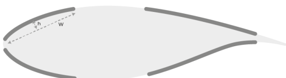
Fig. 3.3: Measurement from the arc of the retrieved element seen in a sectional view.
