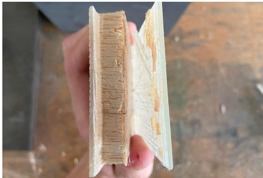
Fig. 4.8: Delamination of laminate itself due to chiselling
