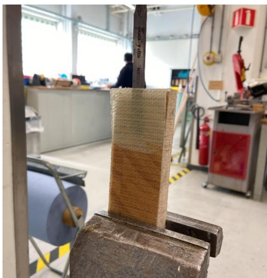
Fig. 4.3: Wedging into the sandwich structure.
