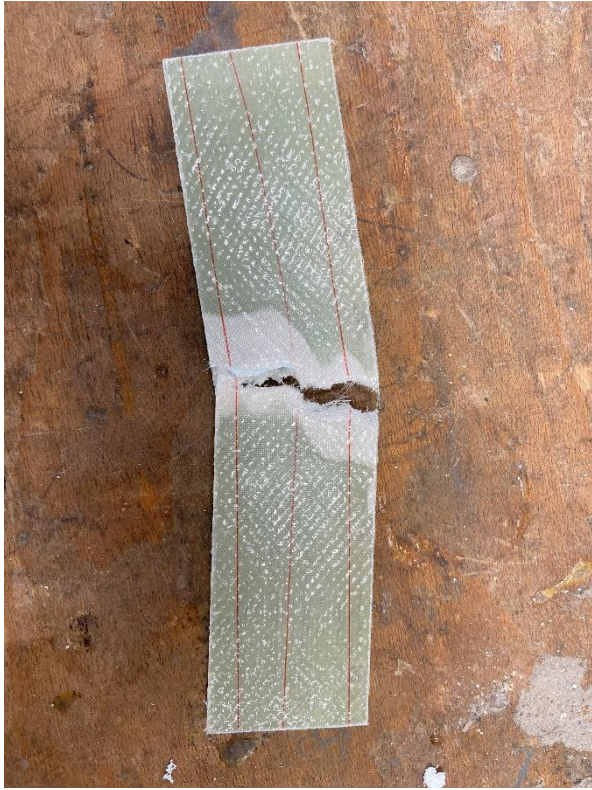
Fig 5.5: broken specimen after bending.
