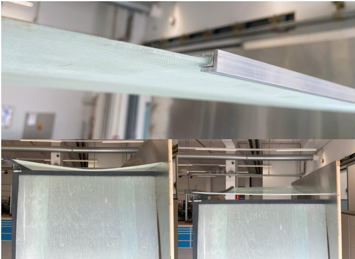
Fig. 8.10: The roof without (buckling) and with the rails
