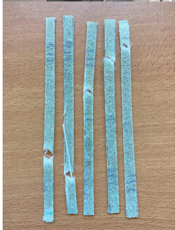
Fig 5.7: A torn GRP specimen
