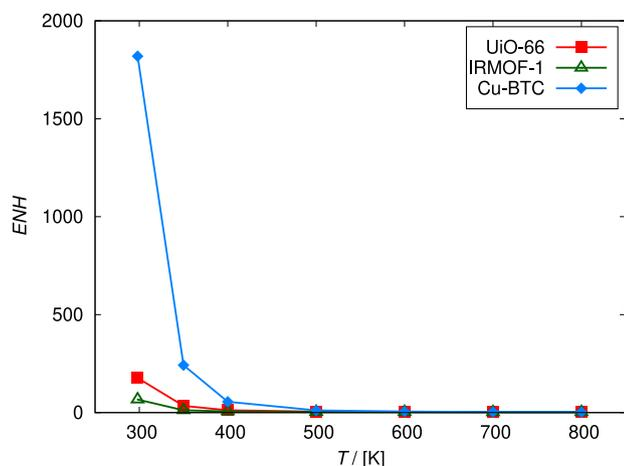
**Fig. 8.** Enhancement ( $ENH$ , Eq. (8)) in the production of HCOOH obtained from GCMC simulations in UiO-66, Cu-BTC, and IRMOF-1 frameworks at 298.15–800 K and 60 bar. The enhancement in HCOOH production resulting from the effect of confinement decreases with increasing temperature. The enhancement in the HCOOH production is the highest in Cu-BTC framework. The obtained mole fraction of HCOOH is 1819 times higher compared to the bulk-phase at 298.15 K.
