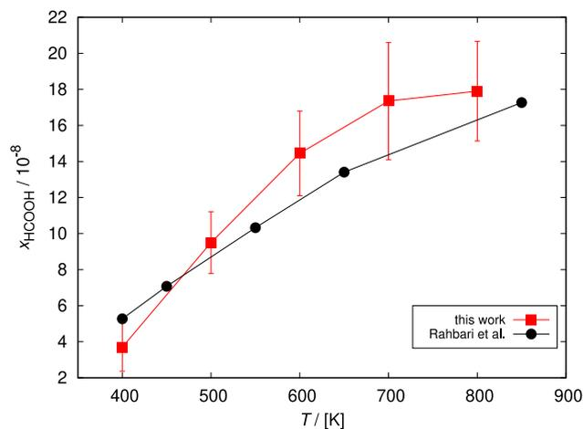
Fig. 1. HCOOH mole fractions computed from the Rx/CFC simulations in the bulk-phase and calculated from equilibrium constants of  $\text{CO}_2$  hydrogenation reaction from the study of Rahbari et al. [71]. The Rx/CFC simulations were carried out at 400–800 K and 1 bar. As the equilibrium constants reported in the study of Rahbari et al. [71] lack uncertainty values, it is assumed that the isobars of simulated and calculated HCOOH mole fractions overlap within the error bars.
