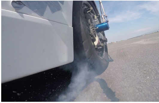
(a) Wheel slip during brake test
