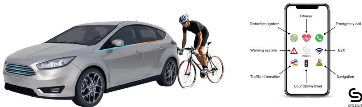
Figure 8.4. The omnidirectional eHMI concept is illustrated with a proximity indicator (left) and the on-bike mobile application CycleSafe (right).
