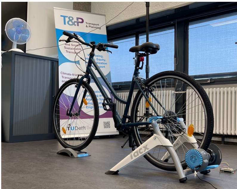
Figure 8.5. The VR cycling simulator (2023) of the Mobility of eXtended Reality lab at Delft University of Technology.
