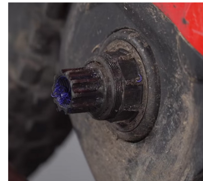
Figure 4.2. Dust and grit around the crank.
