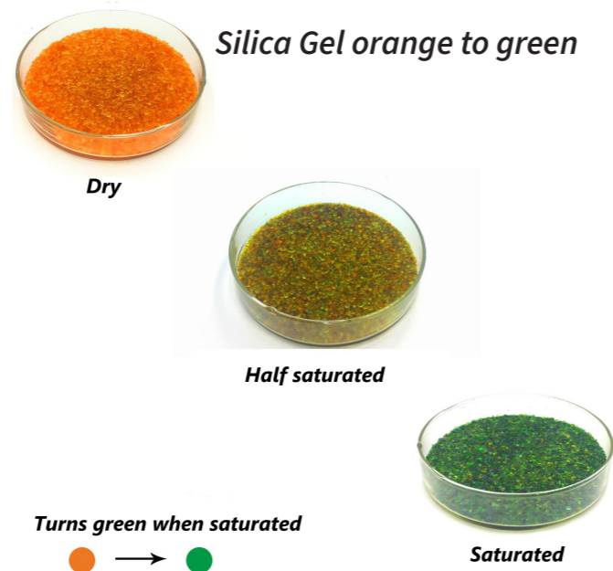
Figure 9.3. Saturation levels of Silica Gel.
