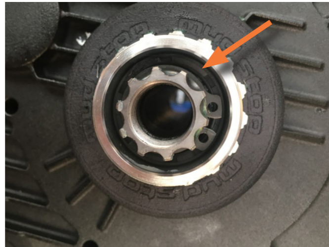
Figure 4.13. Water seal around crankshaft.
