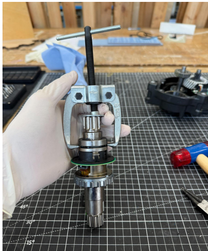
Figure 4.8. Extracting ball bearing with a bearing pulley (left) and fitting with a bearing press (right).
