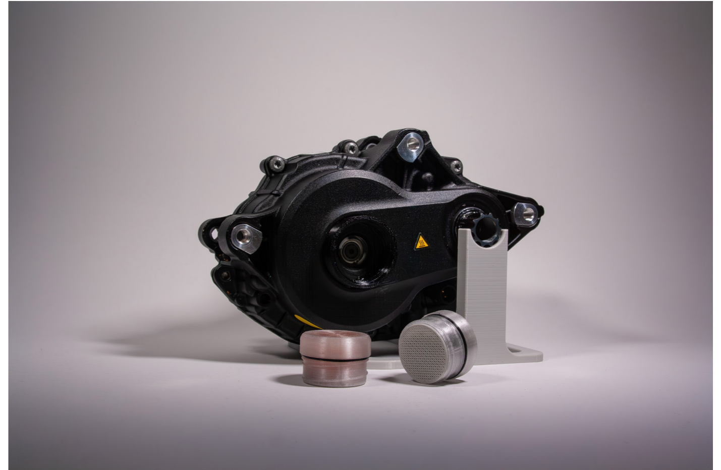
Figure 9.1. Photo of the motor with the desiccant cartridge.
