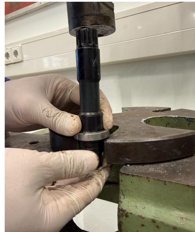
Figure 4.8. Extracting ball bearing with a bearing pulley (left) and fitting with a bearing press (right).
