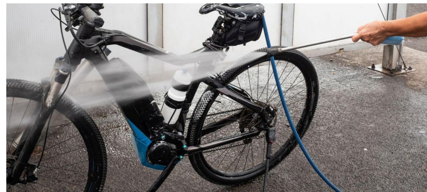
Figure 4.3. Washing an e-bike motor with a pressure washer.
