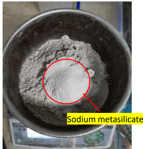
112 113 Fig. 2. Direct addition of sodium metasilicate particles into the dry mixture (GBFS + sand) 114 prior to the addition of distilled water into the system.
