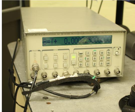
Figure 4.14: Stanford box for synchronised triggering.
