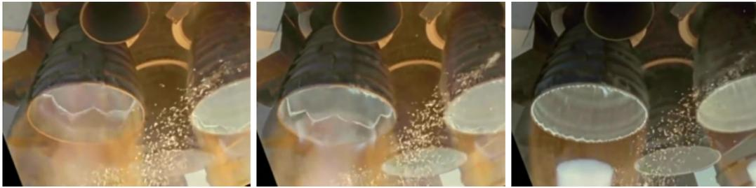
Figure 2.34: Heavy vibrations of the space shuttle main engine during transient start-up due to shock impingement on the flexible wall [73].
