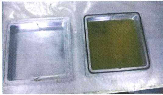
Figure 3-2: The mould used for the clear castings produced with method 2.
