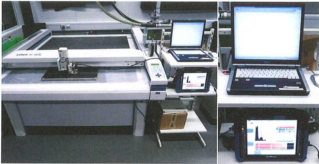
Figure 3-6: The test set-up used during ultrasonic inspection. The ultrasonic flaw detector is connected with a numerical controlled cutting table [19].
