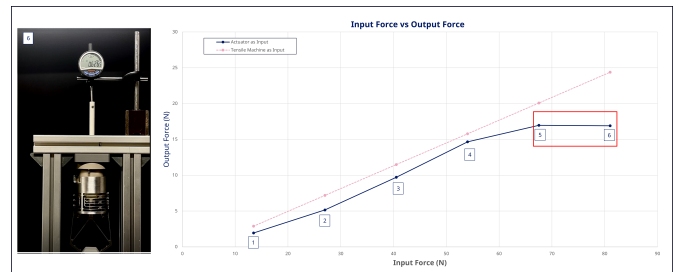
Figure 5.20: Graph with the active gripping results for Instron actuated prototype. And the VCA actuated prototype. The number represent the amount of Amps with which the actuator was powered
