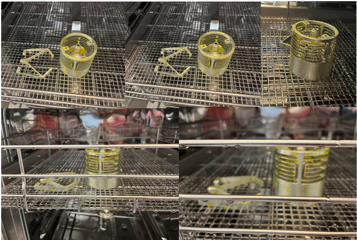
Figure F.7: Coverage test disassembled before wash cycle
