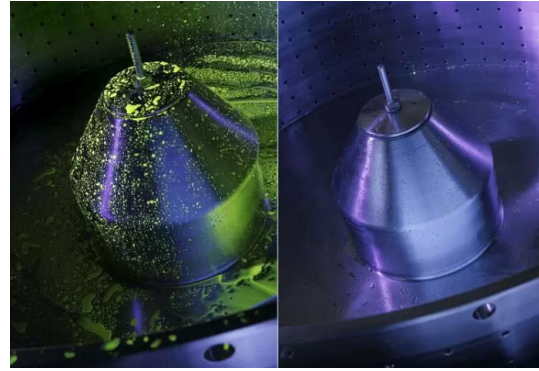
Figure 2.1: An Example of Cleaning Coverage Test Using Riboflavin to Verify Cleanability of Design. Image from [31]
