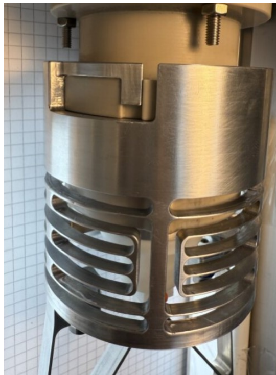
Figure E.3: Engaged snap fit locking mechanism
