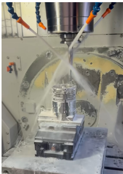
Figure 5.11: CNC production of the LGM prototype out of AL7075
