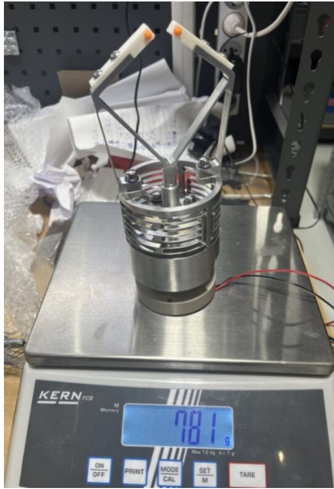
Figure E.5: Final design assembled total weight
