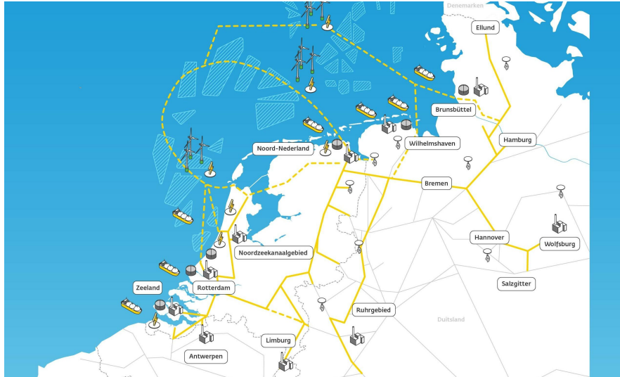
Figure 2.3: Proposed Gasunie hydrogen pipeline infrastructure [1]
