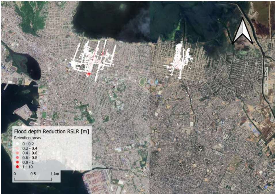
Figure F.16: The reduced flood levels due to Mitigating Option 3 with relative sea level rise imposed.
