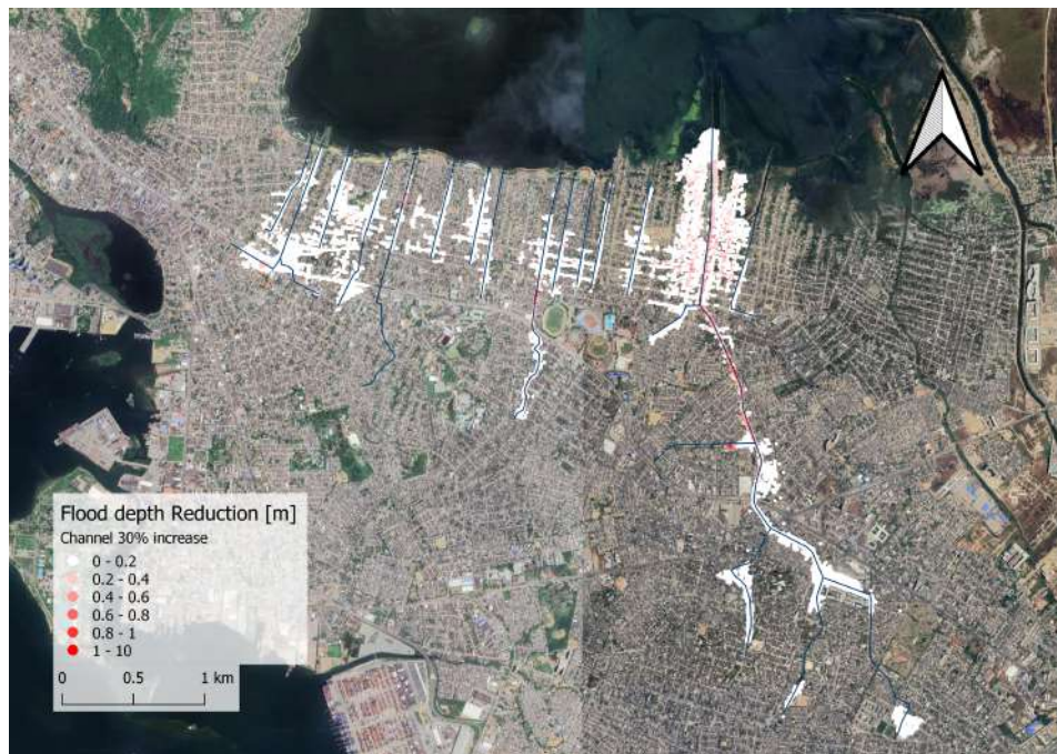
Figure E.6: The flood level reduction with after the increase of 30 % channel width and height.
