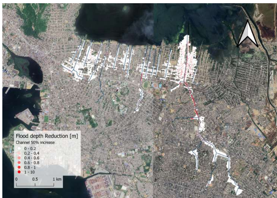
Figure E.8: The flood level reduction with after the increase of 50 % channel width and height.
