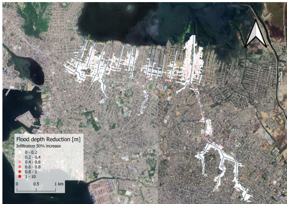
Figure E.22: The flood level reduction after the increase of 50 % of infiltration.
