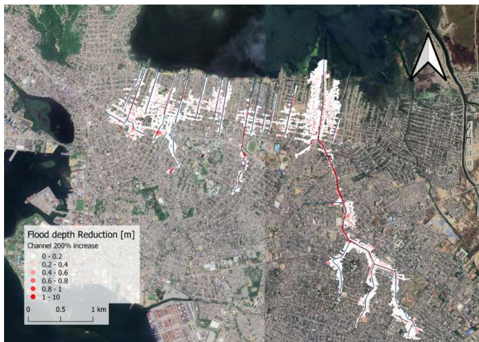
Figure E.12: The flood level reduction after the increase of 200 % channel width and height.
