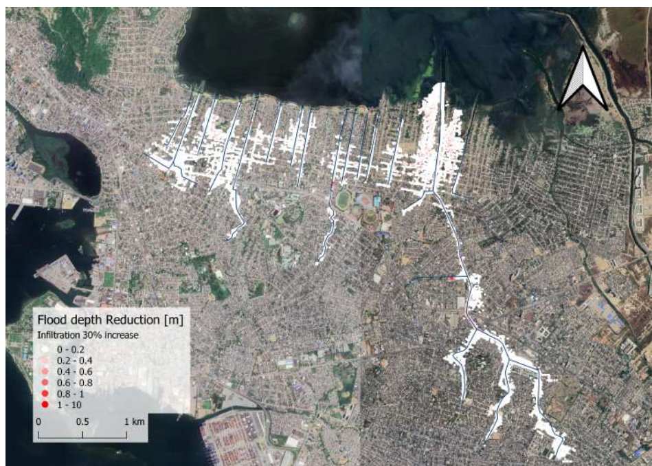
Figure E.18: The flood level reduction after the increase of 30 % of infiltration.
