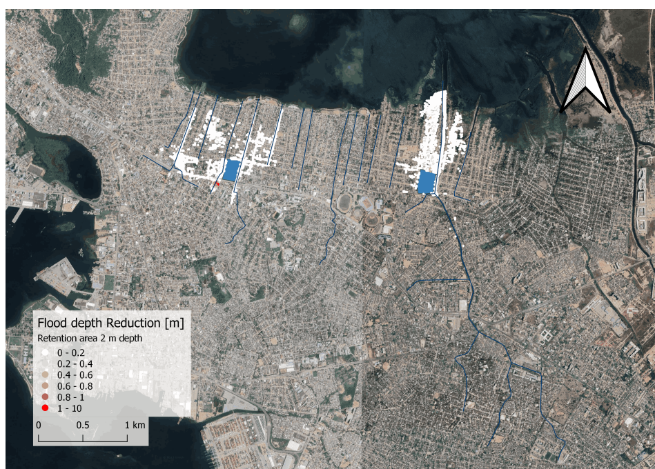
Figure E.24: The flood level reduction after the establishment of two retention areas with a 2-meter depth.
