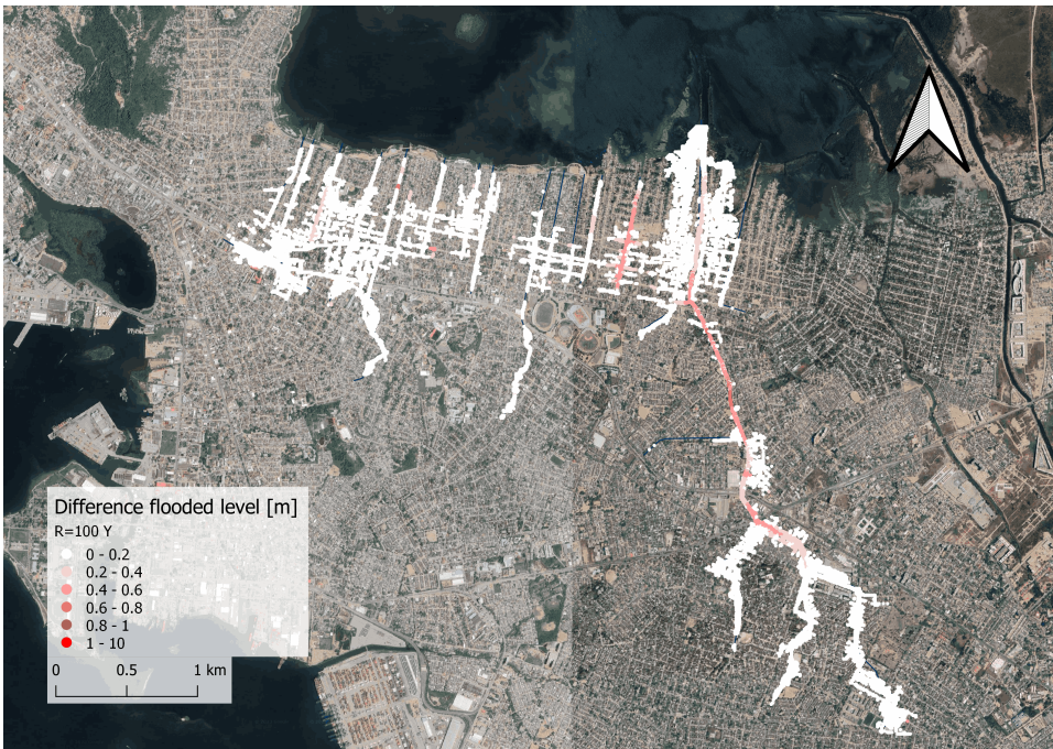
Figure F.2: The increase in flood levels (above 1 mm difference) due to the change of rainfall intensity from R=2 Y to R=100 Y.
