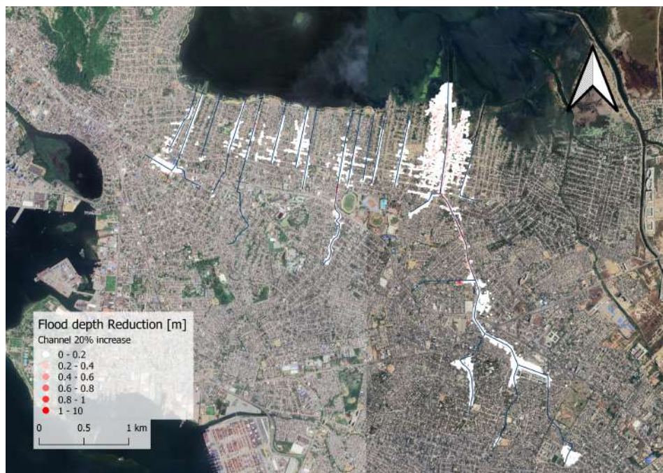
Figure E.4: The flood level reduction with after the increase of 20 % channel width and height.
