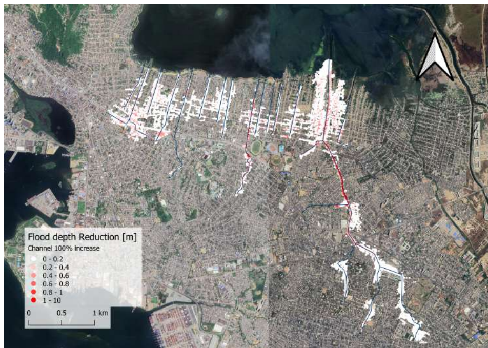
Figure E.10: The flood level reduction after the increase of 100 % channel width and height.
