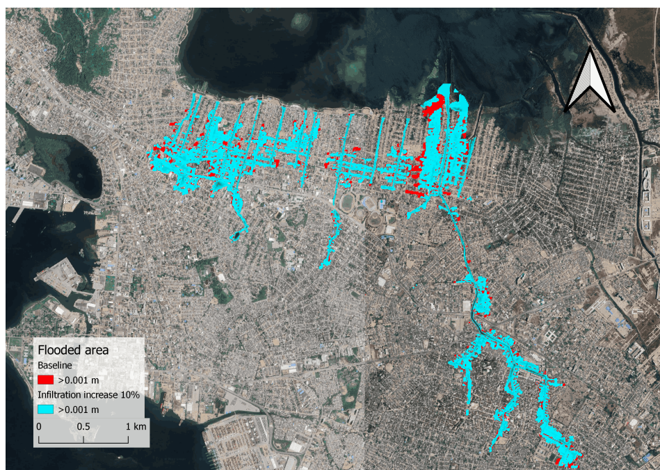
Figure E.13: The reduction in flooded area after the increase of 10 % of infiltration.
