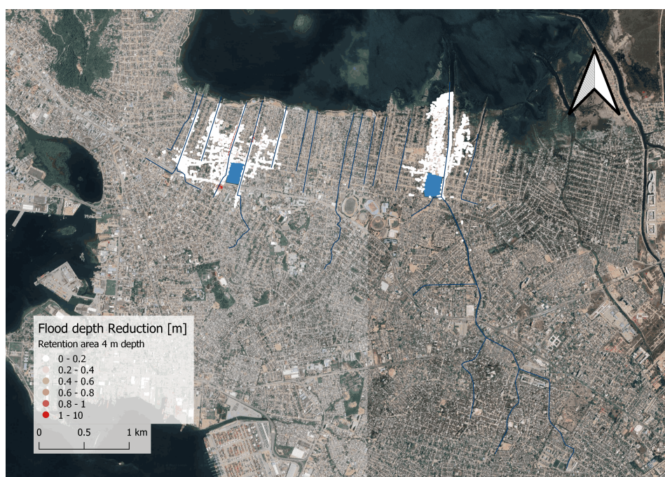
Figure E.26: The flood level reduction after the establishment of two retention areas with a 4-meter depth.
