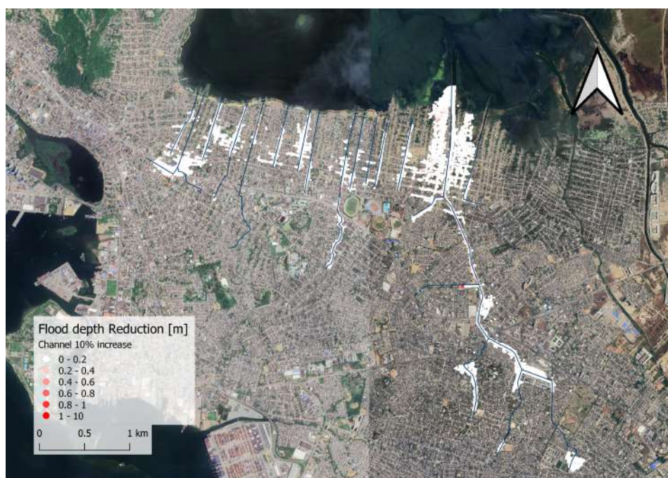
Figure E.2: The flood level reduction with after the increase of 10 % channel width and height.
