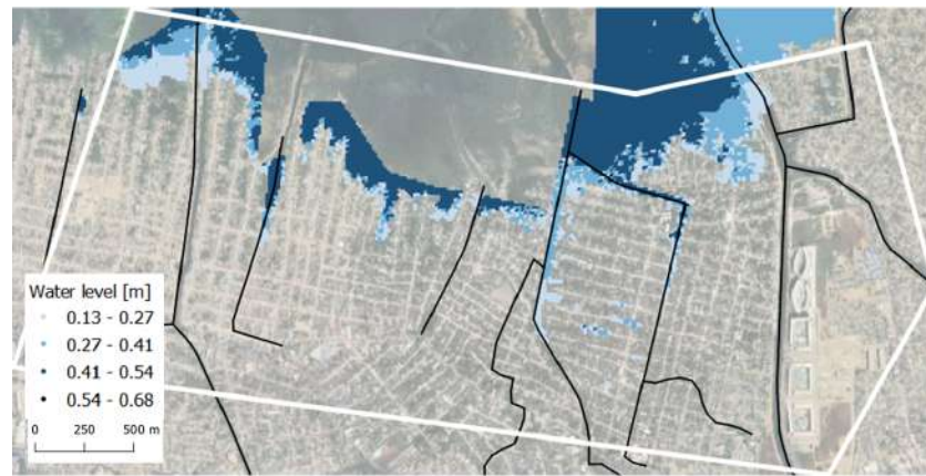
Figure 4.22: The difference in flood levels for extremely high water level and extremely low water level in a scenario with a relative sea level rise. The rainfall intensity in this case has a return period of 100 years
