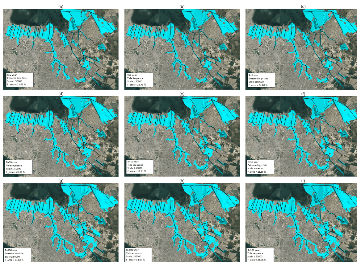
Figure 4.12: (a-c) Rainfall intensity with a return period of 2 years, (d-f) Rainfall intensity with a return period of 10 years, (g-i) Rainfall intensity with a return period of 100 years. (Left column) Extreme low tide, (Middle column) Tidal sequence, (Right column) Extreme high tide
