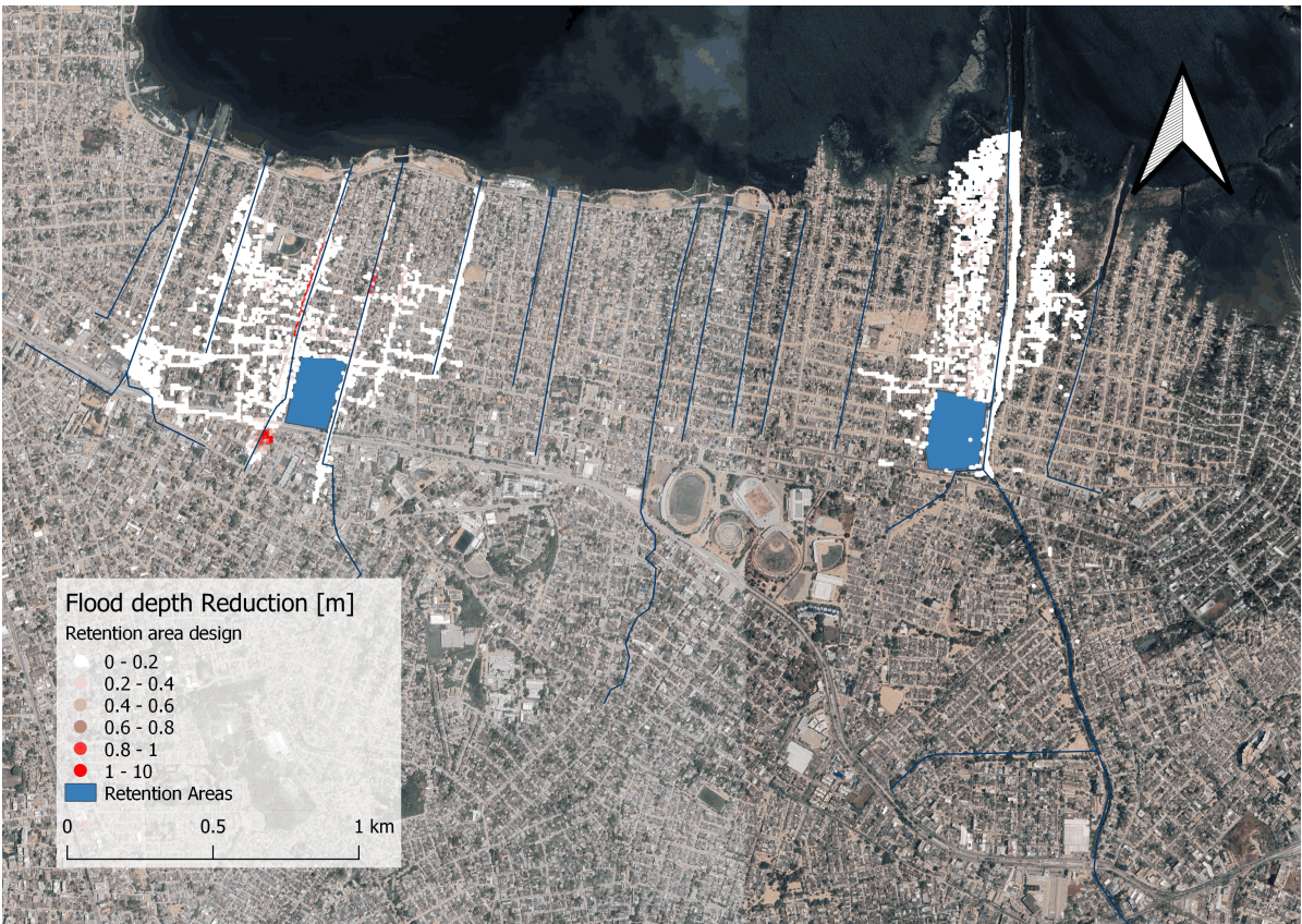
Figure 5.18: The reduced flood levels due to Mitigation Option 3. How redder the dots, how greater the reduction of flood levels.
