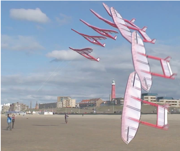
Figure 6.15: A composite representation of the unstable a-symmetric inverted pendulum motion of kiteplane 3.
