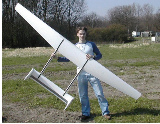
Figure 2.9: An early version of the Kiteplane made from Eperan PP (Poly-Propylene) foam.
