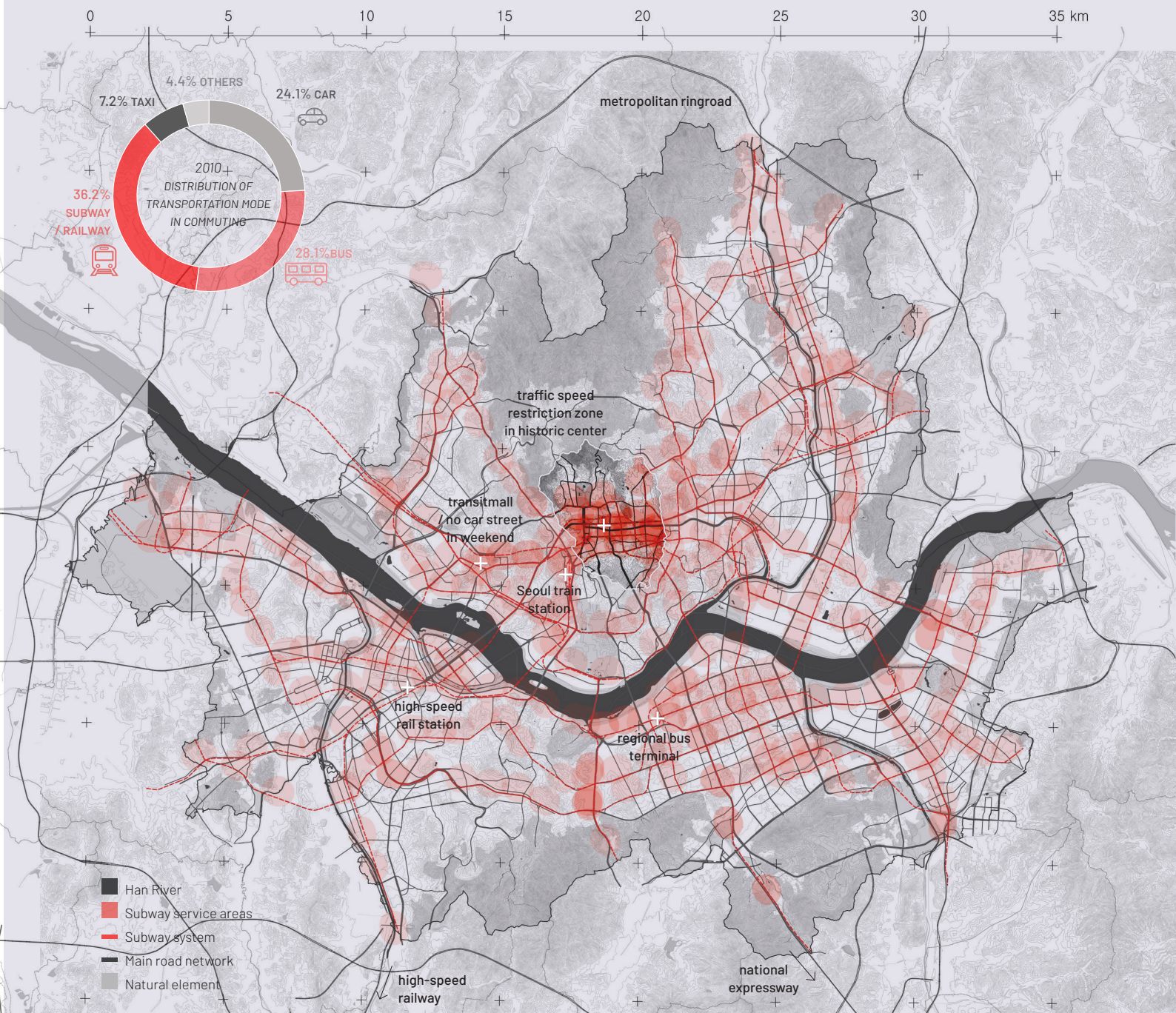
FIG. BOX.1.3 The infrastructure layer of Seoul, showing 500m buffer areas around subway stations.
