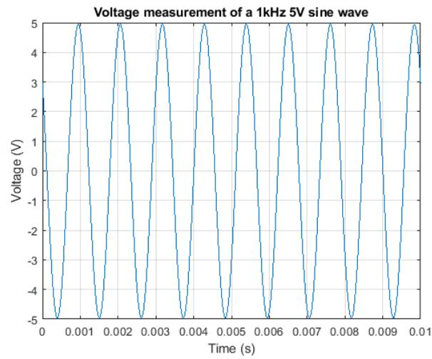
**Figure 8-8:** Voltage measurement of a  $1kHz$ ,  $5V$  sine wave
