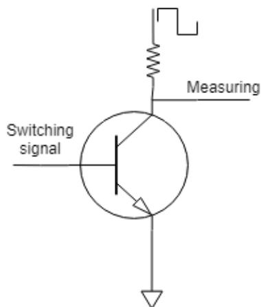
Figure 8-12: Testing circuit for a transistor circuit
