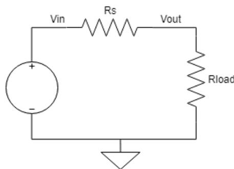
**Figure 8-7:** Voltage divider for current measurement
