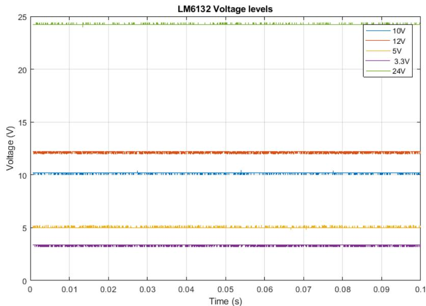
**Figure 6-1:** Bias levels at 3.3V, 5V, 10V, 12V and 24V
