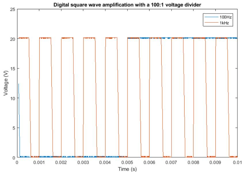
**Figure 6-2:** Square wave of  $100Hz$  and  $1kHz$  with a 100:1 voltage division
