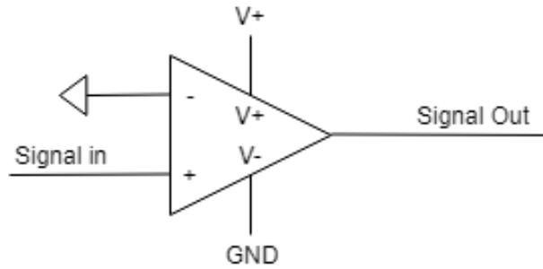
Figure 4-3: Amplifying circuit for digital signals
