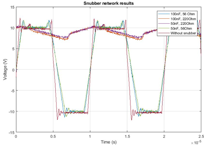
Figure 6-7: Results of a snubber network
