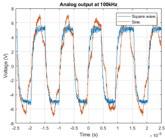
Figure 8-3: Analog outputs at 100kHz
