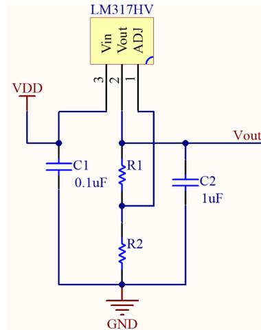
Figure 4-5: LM317HV circuit
