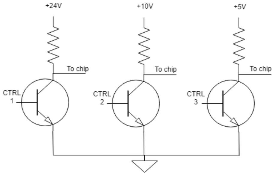
**Figure 3-1:** Transistor network for switching voltages
