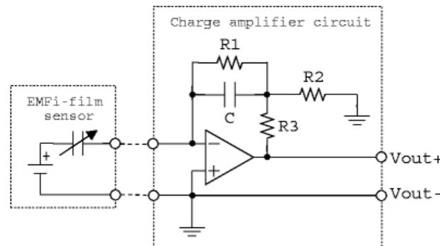
**Figure 1-3:** Circuit film sensor
