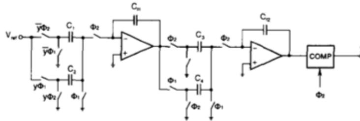
**Figure 1-2:** Second-order capacitor readout circuit
