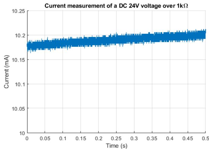
**Figure 8-5:** Measuring of the current of a 24V DC signal through a  $1k\Omega$  resistor
