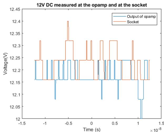
Figure 8-4: 12V DC measured at the socket and at the opamp
