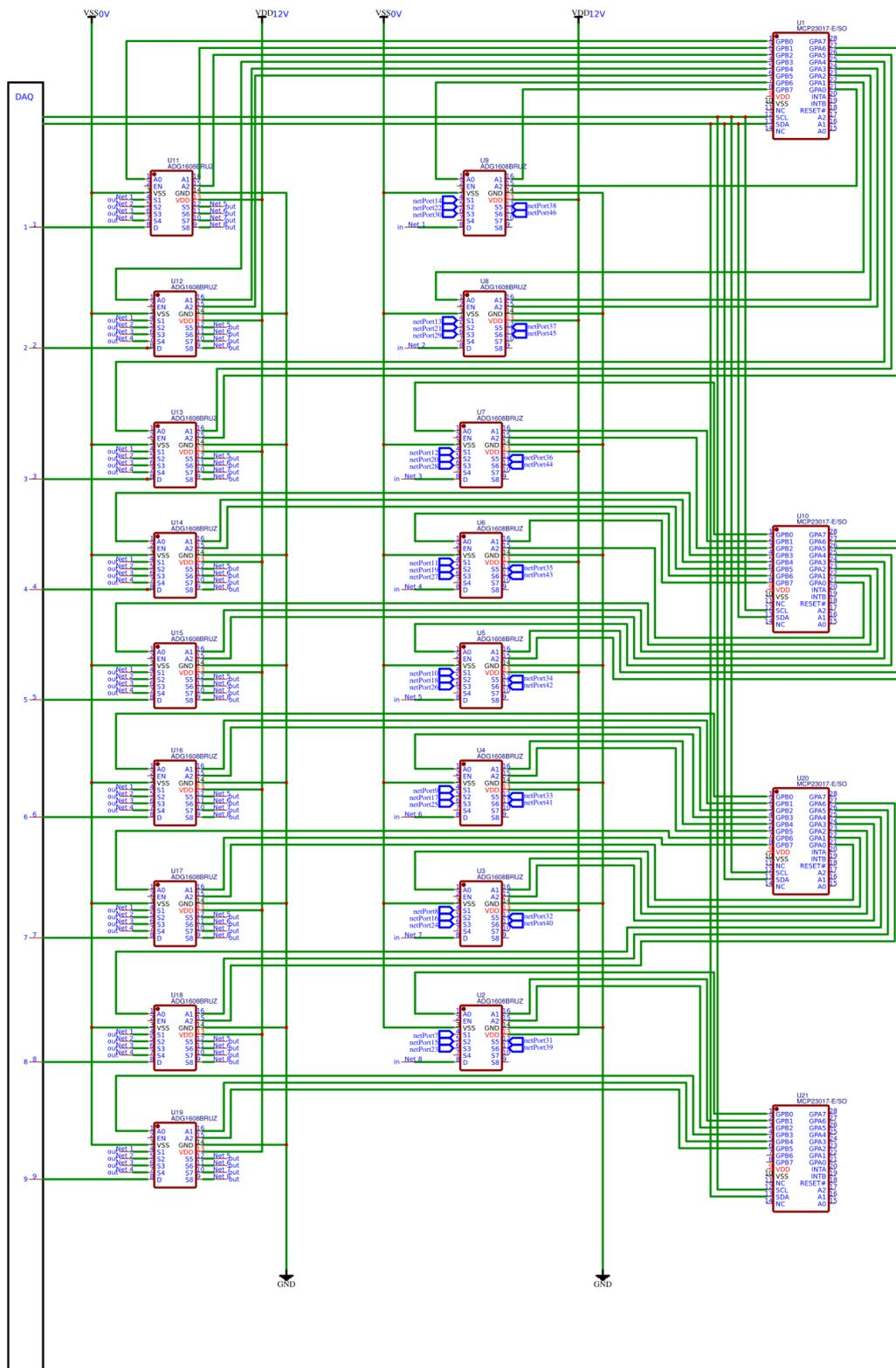
Figure A-2: Multiplexer circuit of the first design
