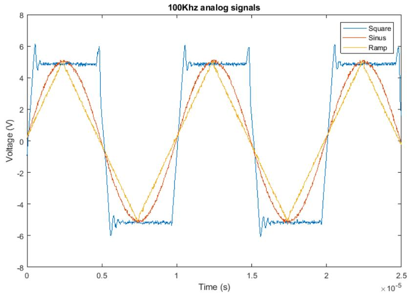
Figure 6-5: 100kHz analog signals
