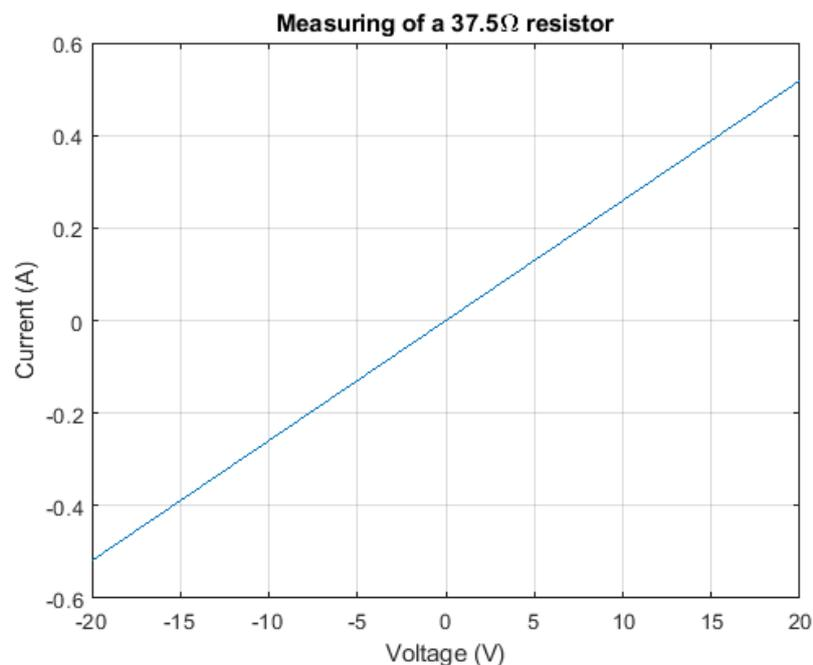
**Figure 8-13:** Test results for a 20V voltage over a 37.5Ω resistor
