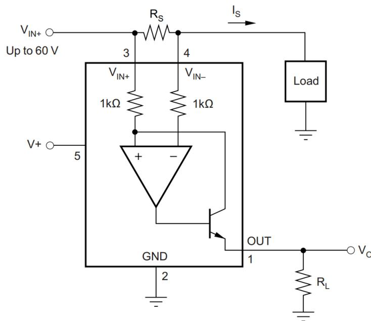
Figure 4-4: Current sensing circuit with the INA169
