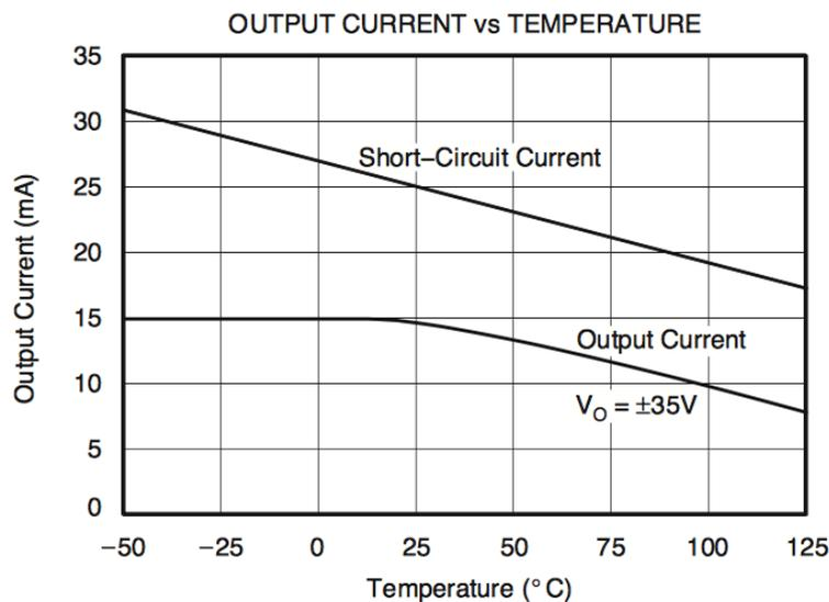
Figure 5-1: Output current vs temperature characteristic for the OPA445
