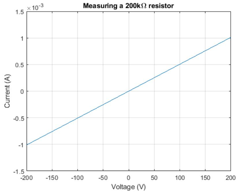
**Figure 8-14:** Test results for a 200V voltage over a 200k $\Omega$  resistor
