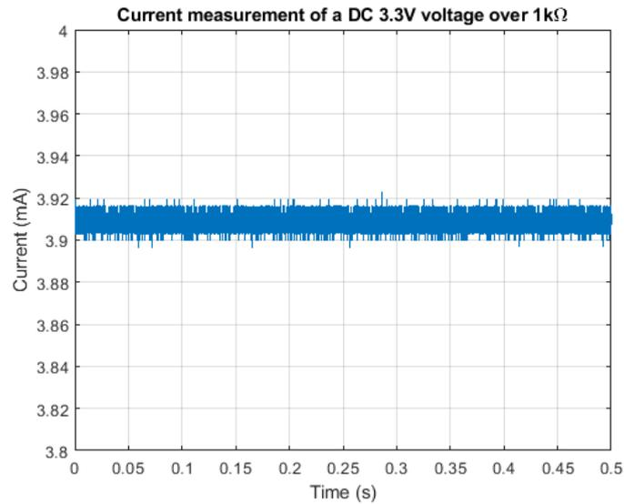
**Figure 8-6:** Measuring of the current of a 3.3V DC signal through a  $1k\Omega$  resistor
