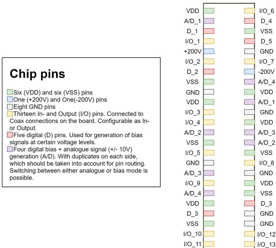
**Figure 7-2:** Pinout for the socket on the PCB
