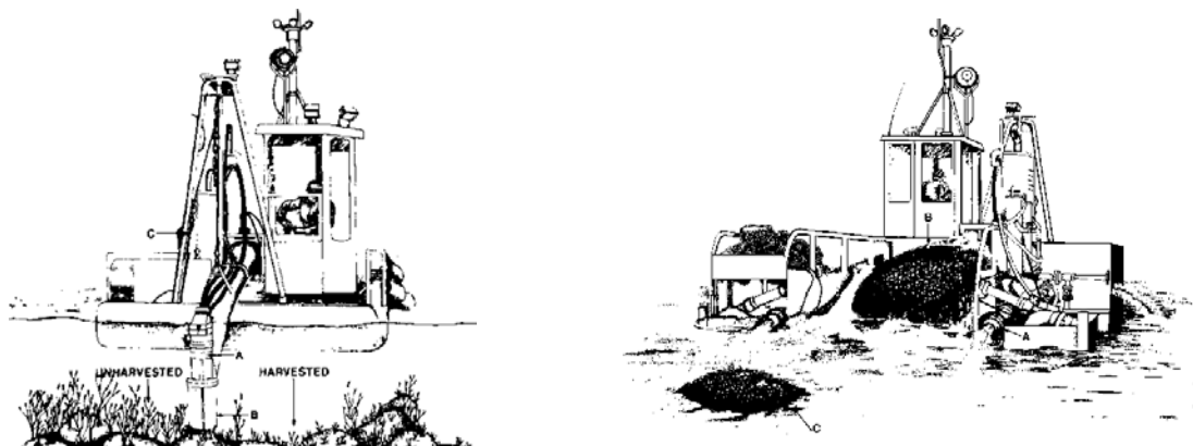
Figure 24 Front and rear view of a Norwegian suction cutter Ascophyllum harvester
