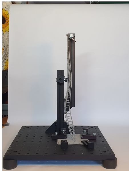
(d) Snap-through scale model exoskeleton at measurement setup.
