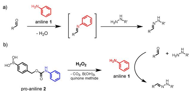
**Scheme 1.** Catalysis of hydrazone formation. (a) Hydrazone formation: the reaction between an aldehyde and a hydrazide catalysed by aniline **1**. (b) The pro-catalyst pro-aniline **2** and the chemical signal H<sub>2</sub>O<sub>2</sub> react to release the organocatalyst aniline **1** which catalyses hydrazone formation between an aldehyde and a hydrazide.<sup>[8]</sup>
