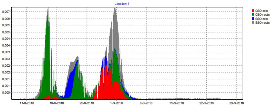
Figure 49 - Overflow fractions at Location 1 in the summer period. The “route” overflows had a maximum fractional contribution of 0.7%.
