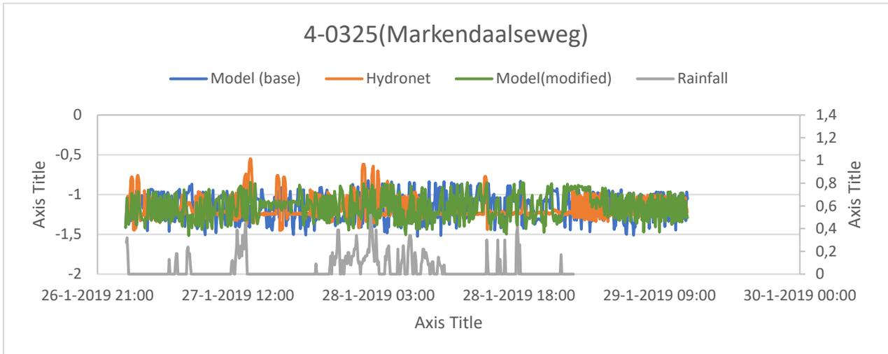
**Figure 17- Simulated and measured water levels at pumping station 4-0325. The measured values corresponded with simulated values.**
