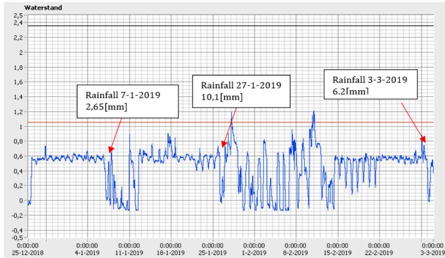
Figure 23 - Measured water level by the sensor at CSO V. The raised water level in dry weather declined after rainfall. An explanation might be light clogging at CSO removed by higher sewer discharges.
