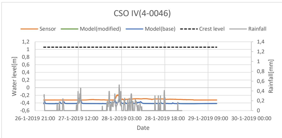
**Figure 21- Simulated and measured water level at CSO IV.**
