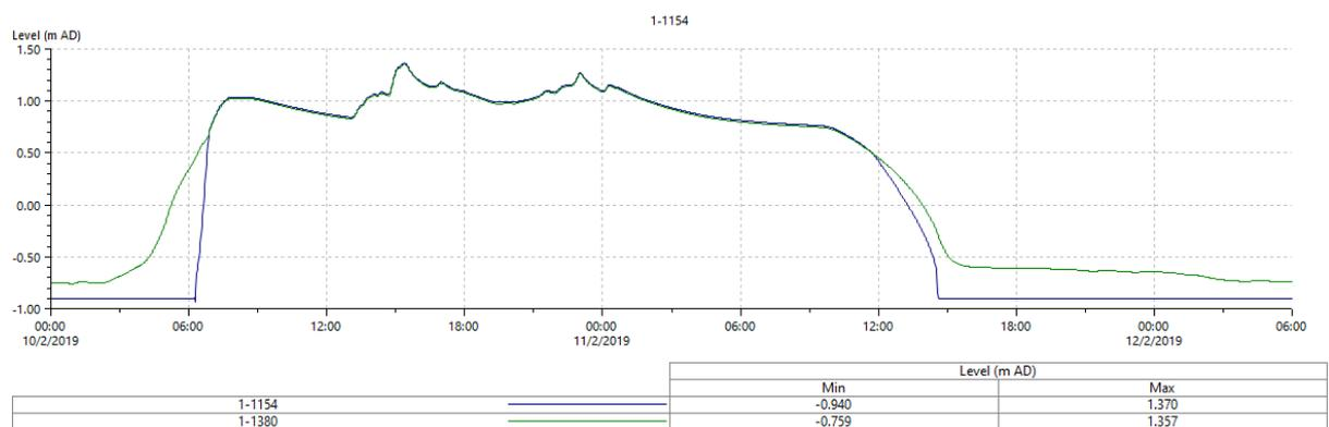
Figure 34- Water level at locations of sensors simulated rainfall on 10-02-2019 by INfoWorks. The discrepancy was under 2 cm since the hydraulic pressure at peak for both is same.
