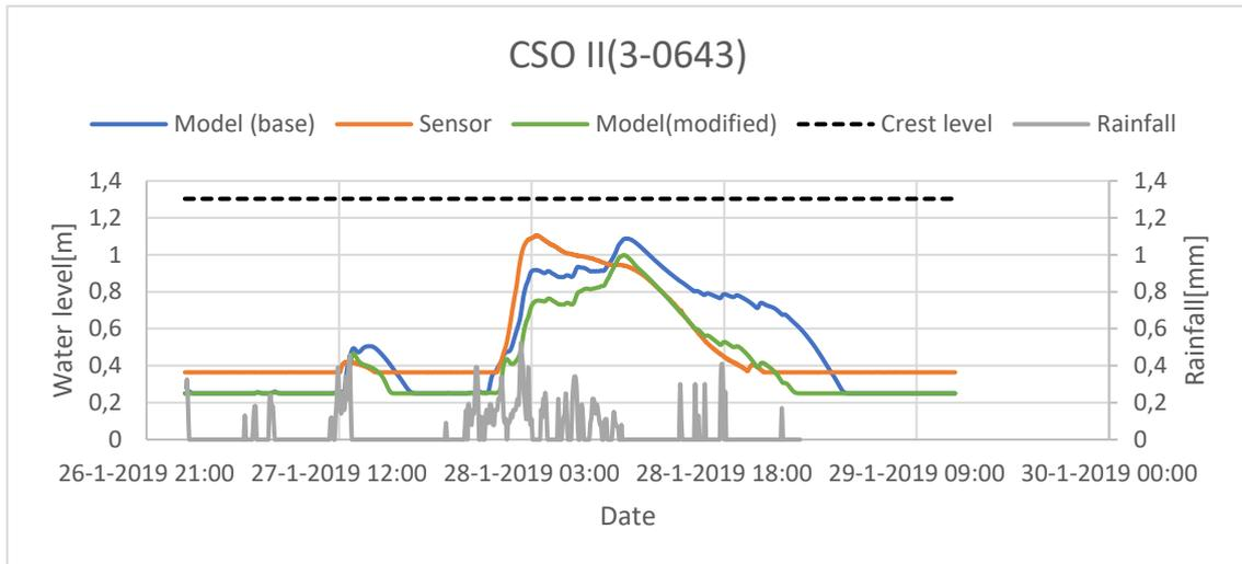
**Figure 19 - Simulated and measured water level at CSO II.**
