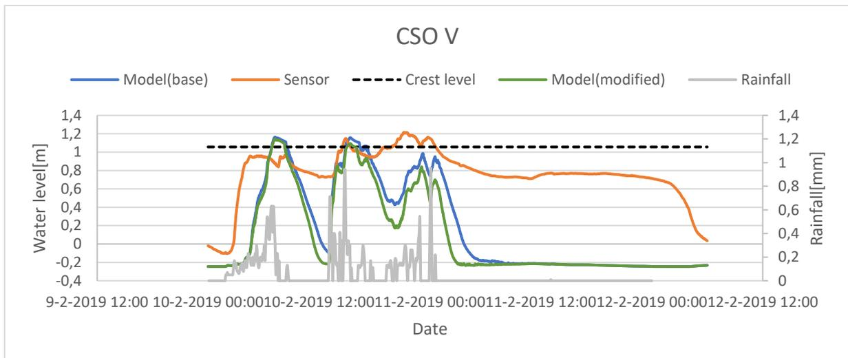
Figure 33-Simulated and measured water levels at CSO V.
