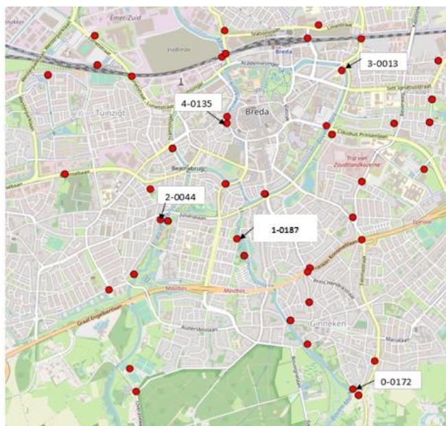
Figure 7 - Selected catchment pump stations, which analysed to clarify the behaviour of the sewer system during rainfall events in context of CSO discharge.
