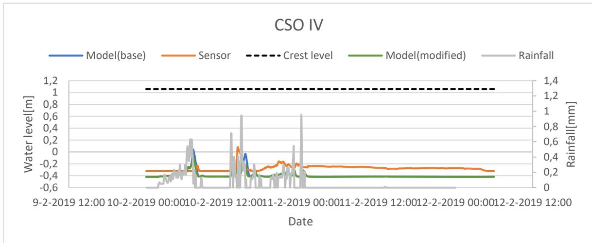
Figure 32-Simulated and measured water levels at CSO IV.
