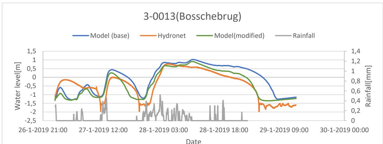
**Figure 16-** Simulated and measured water levels at pumping station 3-0033. The measured values almost corresponded with simulated values.
