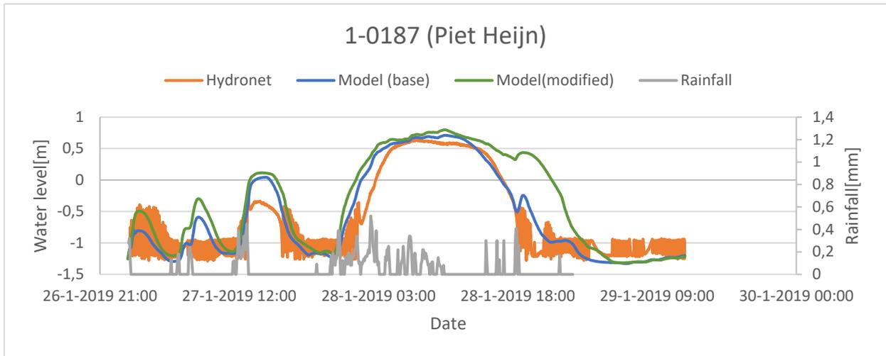
**Figure 14-** Simulated and measured water levels at pumping station 1-0187. The measured values almost corresponded with simulated values. However, the pump capacity was decreased to simulate CSO I discharge.
