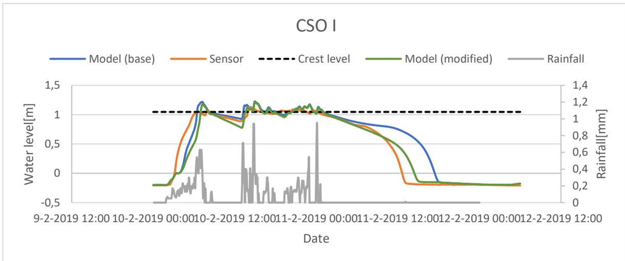
**Figure 29- Simulated and measured water levels at CSO I. The model was modified by decreasing pump capacity to approach CSO discharge. The figure illustrates clearly that by increasing infiltration in modified model, the sewer system received water with delay.**
