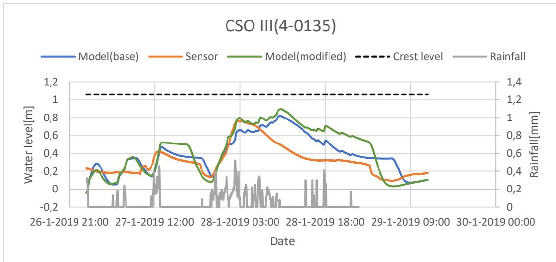
**Figure 20- Simulated and measured water level at CSO III.**
