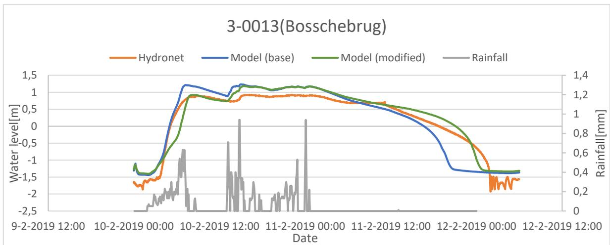
Figure 27- Simulated and measured water levels at pumping station 3-0013.
