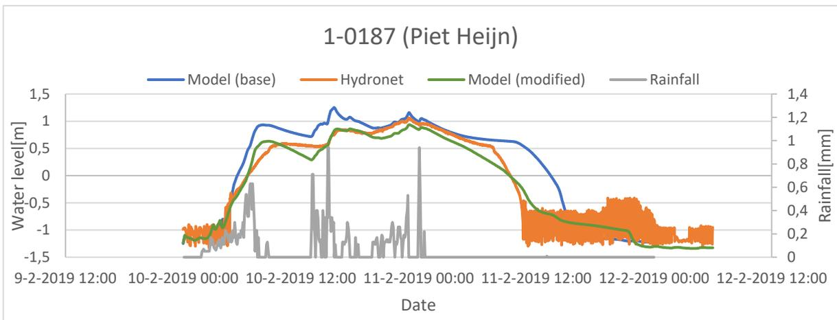
**Figure 25 - Simulated and measured water levels at pumping station 1-0187.**
