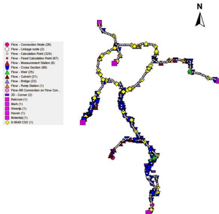
Figure 10 -1D flow model set up for this thesis to simulate water quality based on the Brabantse Delta Waterboard model. In this model, five new boundaries were defined.
