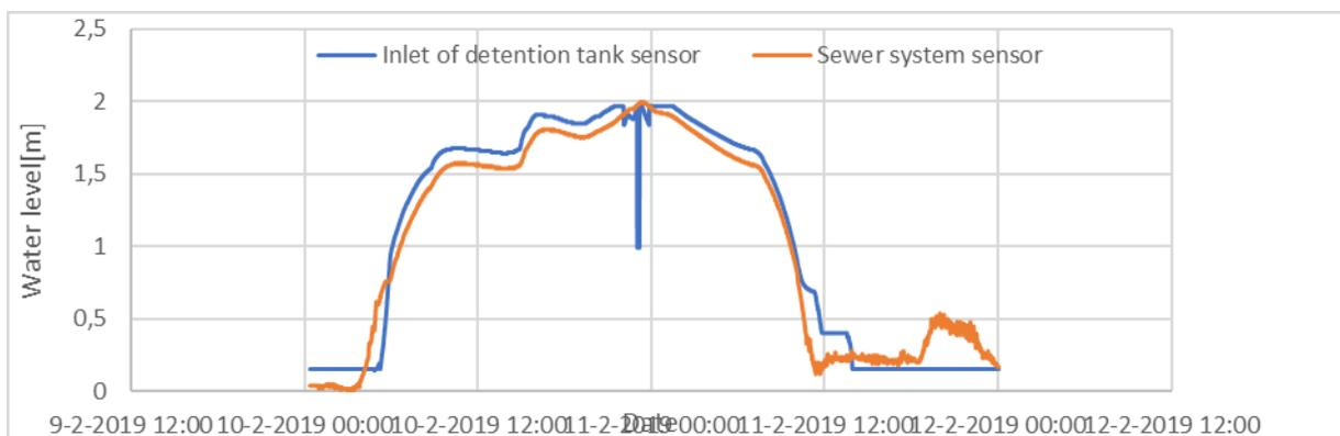
Figure 35- Water levels measured by sensors at both locations of the sewer system within a distance of 300 m and inside the detention tank. The discrepancy is 10 cm, which is considerable. This finding confirms that the level of the sensors might be changed. In addition, an error is detected at CSDT which, can be due the water level reaching a dead zone of the ultrasonic sensor.
