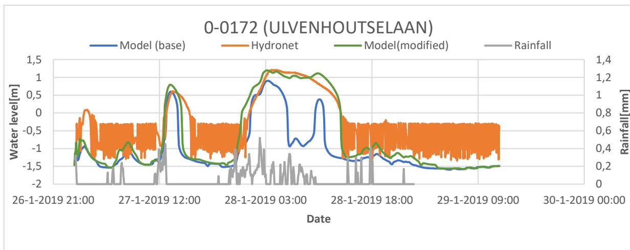
**Figure 13- Simulated and measured water levels at pumping station 0-0172. An explanation for higher measured water levels might be operating pumps with lower capacity due to maintenance work. The model was modified by deleting infiltration factors at catchment 0, 1, 8 and 9.**
