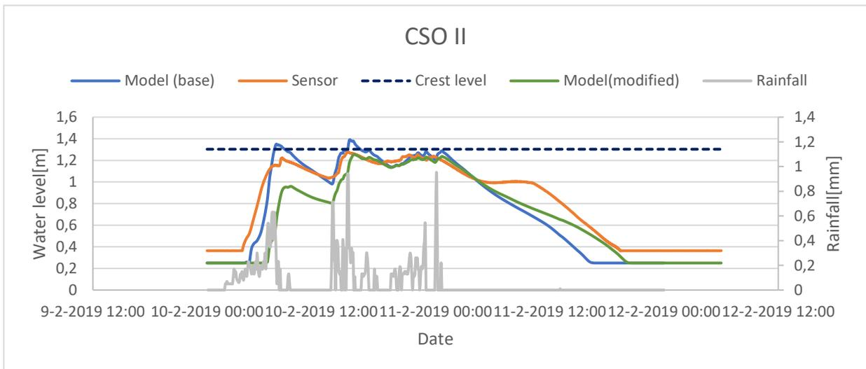
**Figure 30- Simulated and measured water levels at CSO II.**
