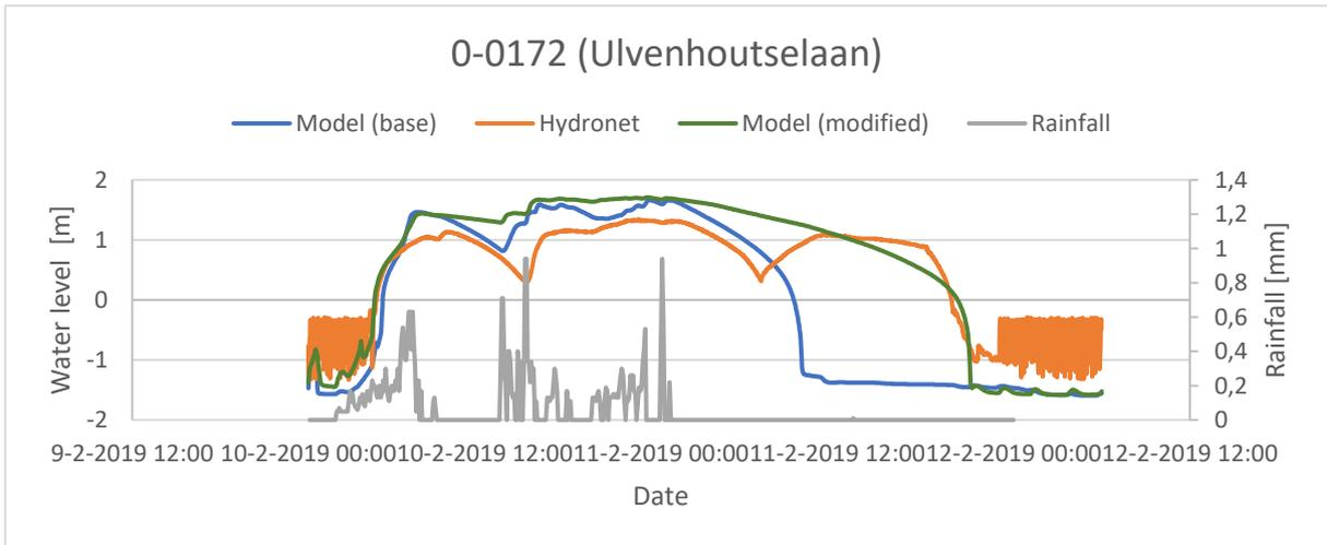
**Figure 24 - Simulated and measured water levels at pumping station 0-0172. The pump was shut off due the maintenance work, thereby taking longer to system be emptied. The model is modified by decreasing pump capacity on 0-0172 and increasing Horton factors at catchments 0, 1, 2, 3, 8 and 9.**
