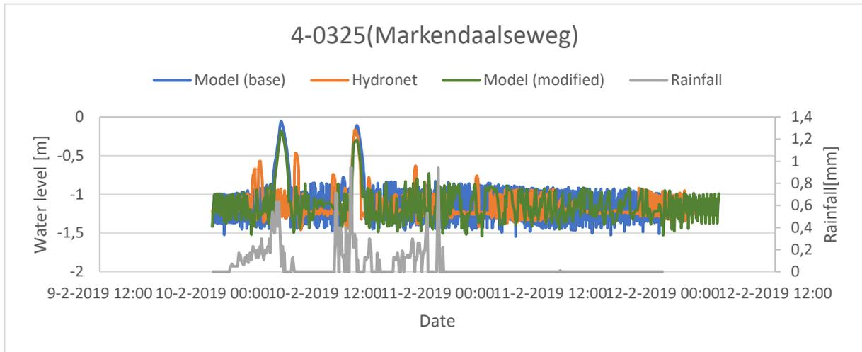
Figure 28-Simulated and measured water levels at pumping station 4-0325.
