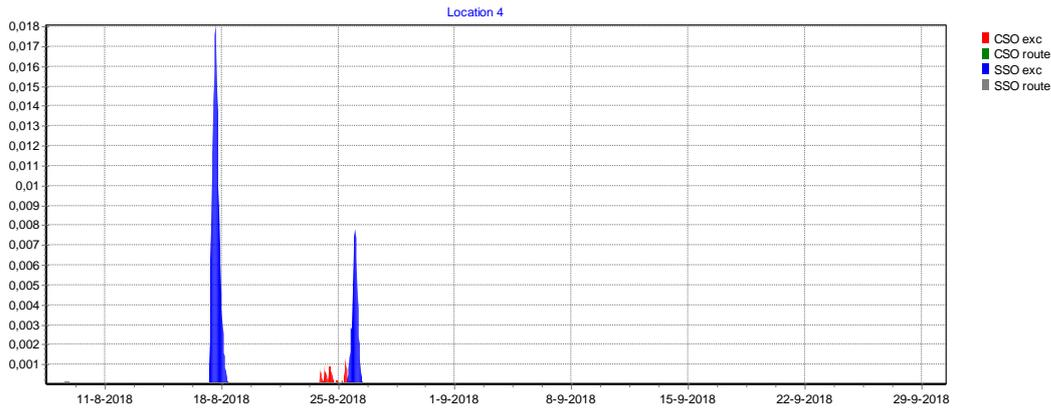
**Figure 40 - Overflows fraction at Location 4 in the summer period. The SSOs of upstream had a maximum fractional contribution of 2%.**
