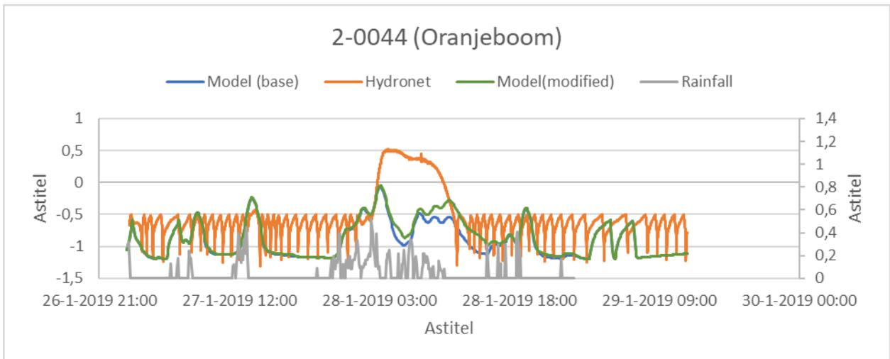
**Figure 15-** Simulated and measured water levels at pumping station 2-0044. The measured values almost corresponded with simulated values. However, the pump capacity was decreased to simulate CSO I discharge.
