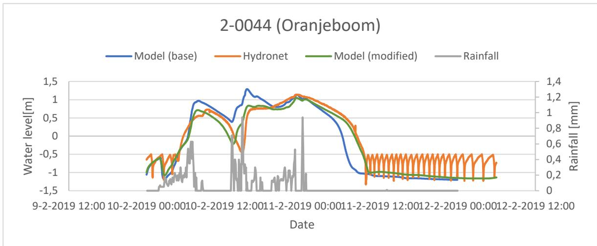
Figure 26- Simulated and measured water levels at pumping station 2-0044.
