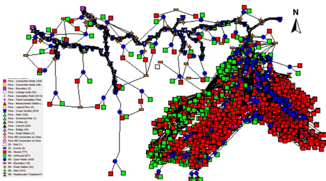
Figure 9 - 1D flow model of the whole water system, which is under supervision of Brabantse Delta Waterboard.
