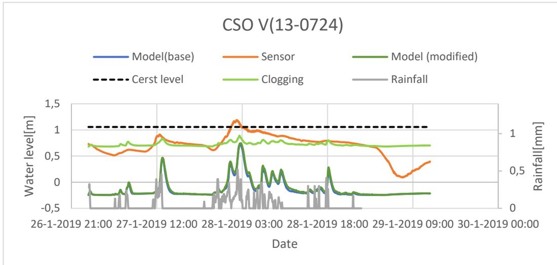
**Figure 22 - Simulated and measured water levels at CSO V. The high water levels in dry weather can be due to clogging removed by rainfall. The plot of simulated clogging in InfoWorks almost corresponds with the measured values.**
