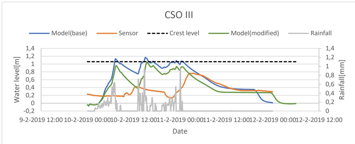
Figure 31-Simulated and measured water levels at CSO III.
