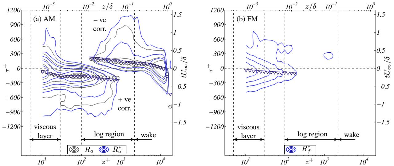
**Figure 1.** (a) Amplitude modulation coefficients as function of phase shift. Lowest level: -0.3, highest level: 0.5 (step 0.1; 0 contour omitted). (b) Frequency modulation coefficient as function of phase shift. Lowest level: 0.1, highest level: 0.4 (step 0.1). A negative phase shift ( $\tau < 0$ ) represents a temporal lead of the small-scale signal with respect to the large-scale signal for a fixed observer.
