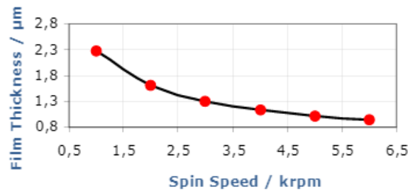
Figure 3.14: Spin curve of AZ ECI 3012 PR [35]
