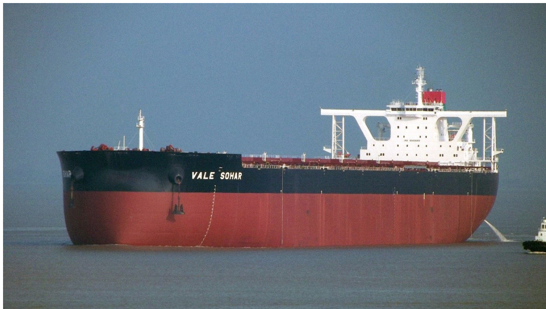
Figure 5.17: The Vale Sohar, a 400,000 DWT dry bulk carrier of the Valemax class (Vale Sohar in Nantong by Dmitriy Lakhtikov is licenced under CC BY-SA 3.0).
