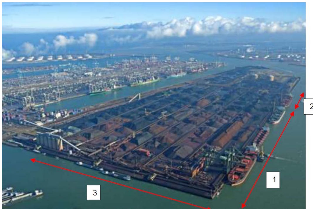
Figure 5.26: EMO-terminal for coal and iron ore, Rotterdam (PIANC, 2019b): (1) large carrier unloading quay; (2) short sea vessel loading quay; (3) barge loading quay.
